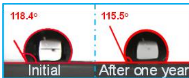
Figure S13. Optical images of water drops on the hydrophobic substrates before and after storage for one year in darkness.
