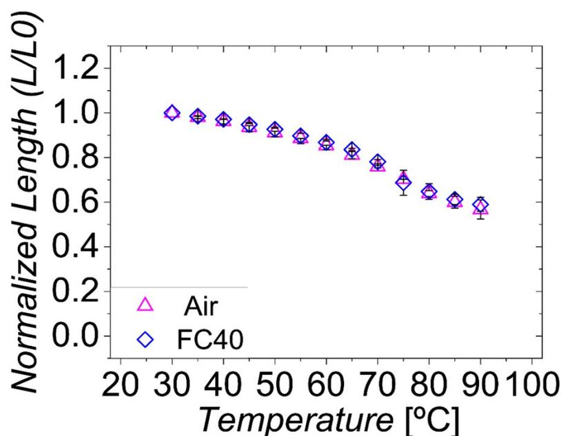
Figure S9. Thermomechanical response in air and FC-40 of uniaxial oriented LCEs ( $65 \pm 5 \mu\text{m}$  thick) with the director along its long axis. A load of 1 g attached to the extreme of the samples is lifted upon actuation. Normalized length ( $L/L_0$ ) of the LC elastomers during the heating from 30 °C to 90 °C. Mean $\pm$ SD of two samples.
