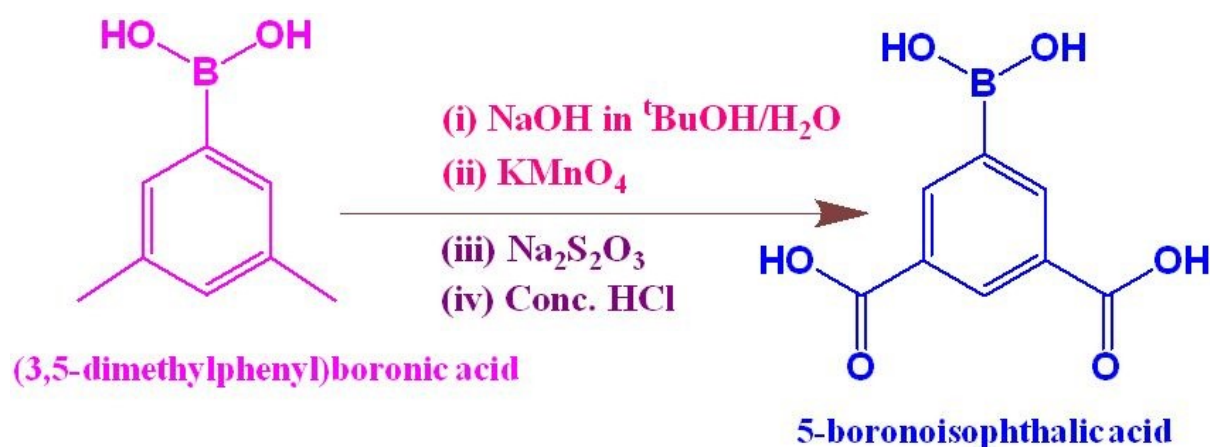
Scheme S1. Reaction scheme for the preparation of 5-boronoisophthalic acid linker.
