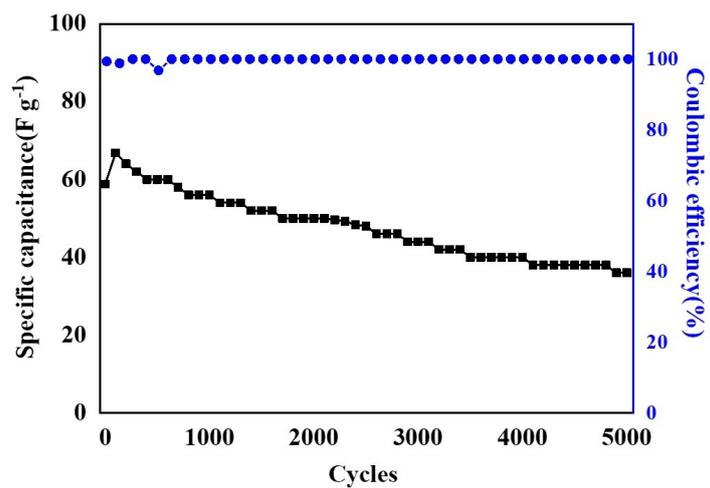
**Fig. S9.** Cyclic performance of the  $\text{Ni}_x\text{S}_6/\text{Ni}(\text{OH})_2//\text{AC}$  asymmetric supercapacitor at a constant current density of  $4 \text{ A g}^{-1}$ .
