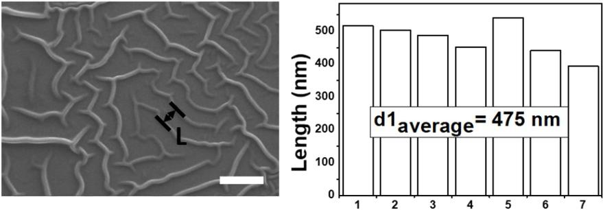
**Fig. S5.** The SEM images show the labyrinth and generating a 1D array of periodic wrinkles with a periodicity of  $L \approx 500 \mu\text{m}$ . The scale bar is 1  $\mu\text{m}$ .
