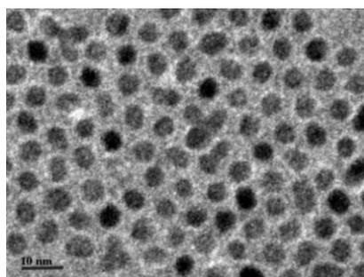
**Fig. S3.** TEM image of individual PEG-coated Fe<sub>3</sub>O<sub>4</sub> nanoparticles.
