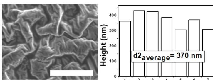
**Fig. S2.** SEM images showing labyrinth pattern and the thickness. The scale bar is 500 nm.
