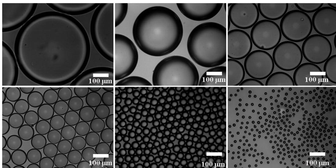
**Fig.S1.** Optical microscopy images showing the different size of microgels by adjusting the outer flow rate and inner flow rate. The scale bar is 100 μm.
