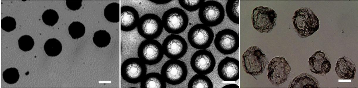
**Fig.S4.** Physical appearance of topographically heterogeneous micromaterials of Optical microscopy images in different assembly conditions. (a) Solidified structure of pure MNPs droplets without BCP, (b) pickering structure show pure BCP without MNPs, (c) Janus structure show 30 wt% MNPs and BCPs. The scale bar is 100  $\mu\text{m}$ .
