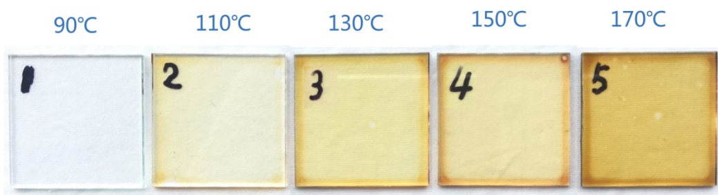
Figure S2. Photograph of the PAMPSA/PVA films coated on the quartz substrates according to the thermal treatment temperature (90–170 °C, 30 min).
