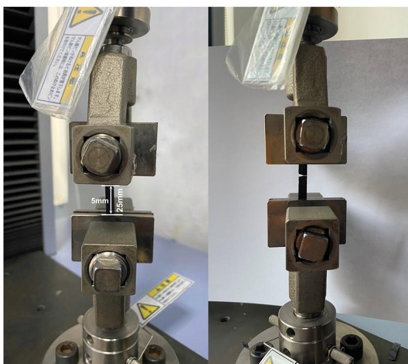
Figure S6. Photographs of a MXene/QCS membrane before a) and after stretching b) under the action of tension machine.
