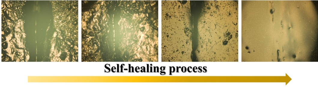
Fig. S11. Digital images of the incision in the self-healing process.
