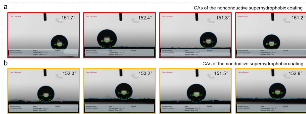
Fig. S8. The water contact angles of the nonconductive superhydrophobic coating and the conductive superhydrophobic coating. (a) The water contact angles of the nonconductive superhydrophobic coating at different locations, showing an average angle of 151.2°. (b) The water contact angles of the conductive superhydrophobic coating at different locations, showing an average angle of 152.3°.
