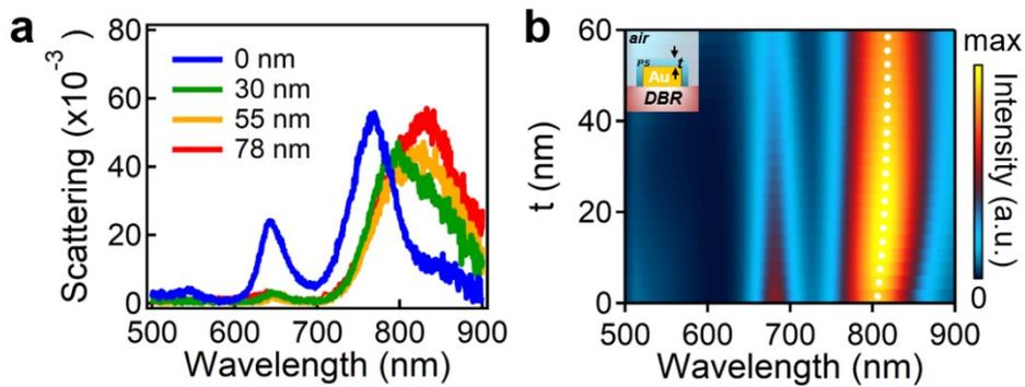
**Fig. S6.** Influence of the dielectric coating on the scattering spectra of Au NPIs-DBR hybrid structures. (a) Scattering spectra of Au NPIs on DBR coated with PS layer of different thicknesses. (b) Simulated dark field scattering spectra of Au NPIs on DBR with different thickness of PS coatings.
