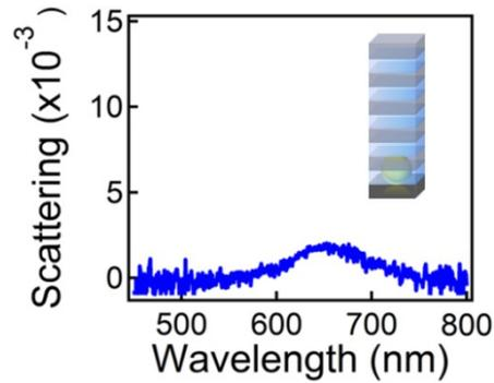
**Fig. S5.** Dark field scattering spectrum of Au NSphs (80 nm) underneath the DBR. The split peaks disappear with one broad scattering peak.
