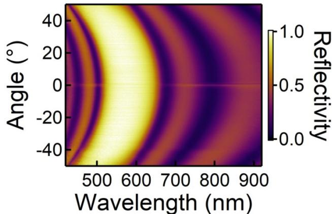
**Fig. S4. Angle resolved reflectivity spectroscopy of DBR samples.**
