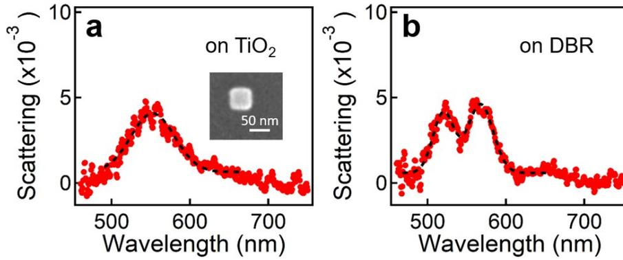
**Fig. S8. Narrowed plasmonic peaks of Au NCs-DBR hybrid structures.** Scattering spectra of 50 nm Au NCs on (a) TiO<sub>2</sub>/Si (inset is the SEM image of the Au NCs) and (b) DBR substrate.
