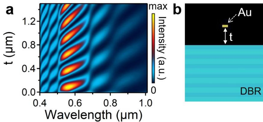
**Fig. S7.** Simulations of Au NPIs on top of DBR with different spacing. (a) Change of scattering spectra with separation between Au NPIs and the DBR. (b) Schematic of the simulated structure. The  $t$  denotes the distance between Au NPIs and DBR surface.
