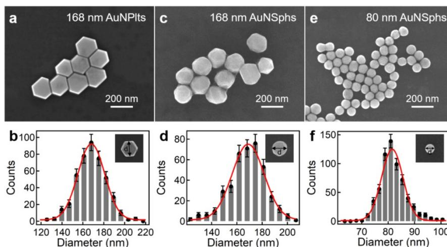
**Fig. S1. Characterizations of the Au NPs used in this paper.** SEM images of (a) Au NPIs, (c) Big Au NSphs, (e) Small Au NSphs and corresponding diameter distributions of (b) Au NPIs ( $168 \pm 16$  nm), (d) Big Au NSphs ( $168 \pm 14$  nm), (e) Small Au NSphs ( $81 \pm 6$  nm).
