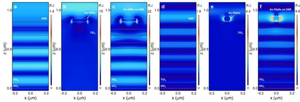
**Fig. S2. Near field simulations.** The simulated E-field distributions of (a) DBR substrate only, Au NPls on (b)  $\text{TiO}_2$  substrate, and (c) on DBR substrate. The dashed lines represent the layer interfaces of DBRs and Au NPls. Excitation wavelength: 728 nm. (d) DBR, Au NSphs on (e)  $\text{TiO}_2$ , and (f) Au NSphs on DBRs. The dashed lines represent the layer interfaces of DBRs and Au NSphs. Excitation wavelength: 530 nm.
