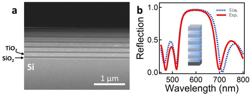
**Fig. S3. Characterization of DBR.** (a) SEM image of DBR cross section and (b) corresponding reflection spectrum at normal incidence angle (Red solid line). Dashed line represents the simulated reflection spectrum which agrees quite well with experiments.
