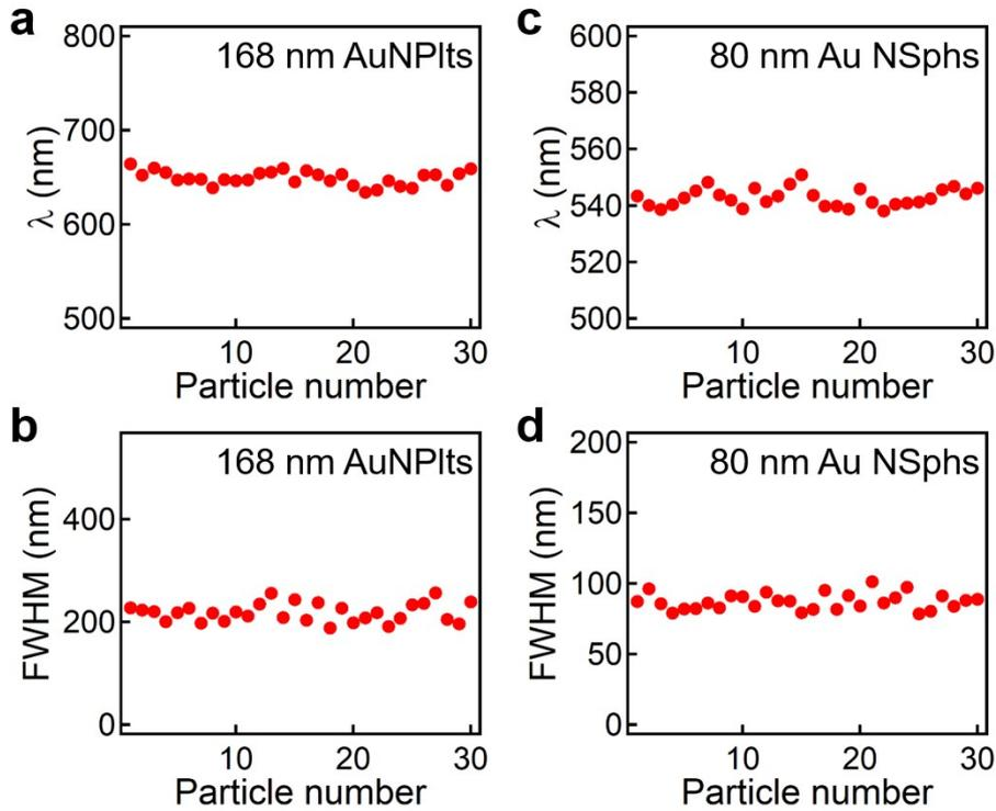
**Fig. S9. Statistics of plasmonic resonances and FWHMs of different NPs.** (a) Plasmonic resonances and (b) FWHM of Au NPIs on TiO<sub>2</sub> substrate, where  $\lambda = 649 \pm 8 \text{ nm}$ ,  $FWHM = 218 \pm 18 \text{ nm}$ . (c) Plasmonic resonances and (d) FWHM of Au NSphs on TiO<sub>2</sub> substrate, where  $\lambda = 543 \pm 4 \text{ nm}$ ,  $FWHM = 87 \pm 6 \text{ nm}$ .
