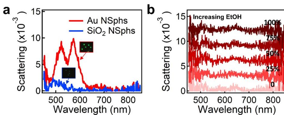
Fig. S11. Scattering spectra and sensing performance of SiO<sub>2</sub> NSphs-DBR hybrid structures. (a) Scattering spectra of Au NSphs (80 nm) and SiO<sub>2</sub> NSphs (80 nm) on DBR. Insets are their DF image. (b) Scattering spectra of SiO<sub>2</sub> NSphs (240 nm) on DBR with increasing amount of EtOH.
