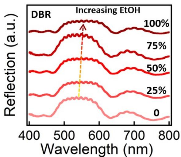
Fig. S10. Sensing measurement based on DBR. Change of reflection spectra of DBR with increasing amount of EtOH.
