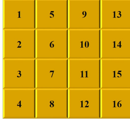
Fig. S6. Schematic diagram of the position number of the 4 \times 4 sensor array
