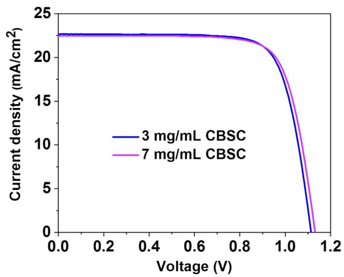
**Figure S3.** J-V curves of 3 mg/mL and 5 mg/mL CBSC passivated perovskite devices.
