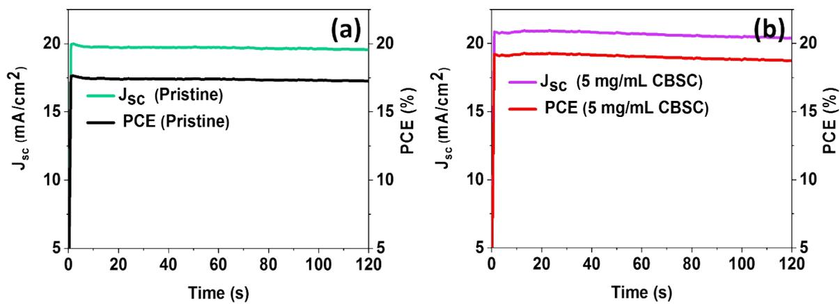
**Figure S5.** The stabilized PCE at the maximum power point (MPP) of a) the pristine device and (b) the CBSC passivated device.
