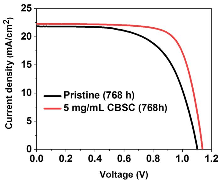
**Figure S6.** J-V curve of pristine and CBSC passivated devices after storing in a dried box (30% humidity and room temperature) for 768 hours.
