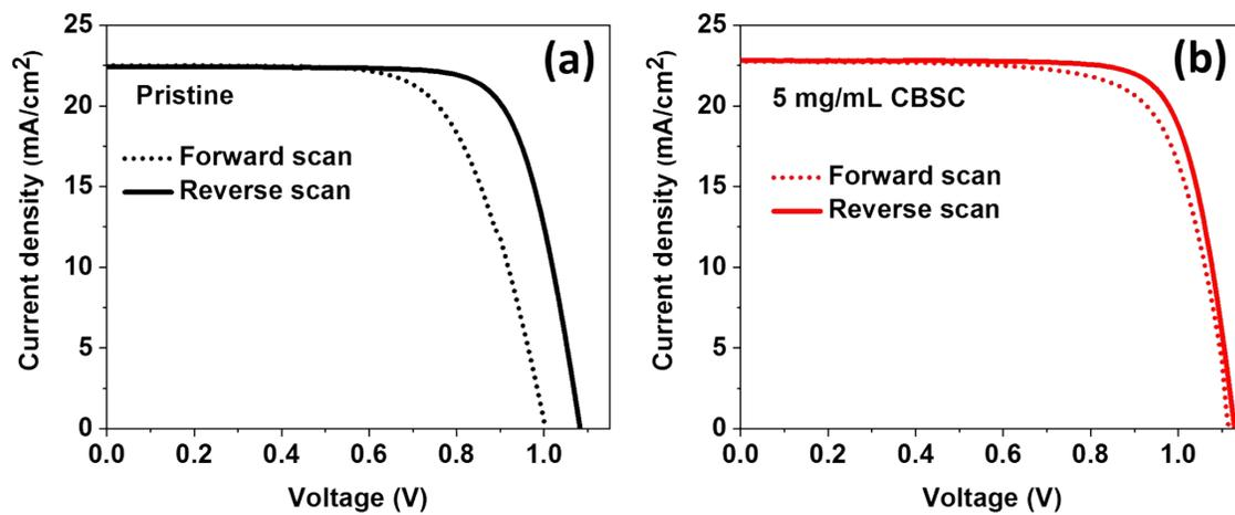
**Figure S4.** J-V curve of (a) the pristine and (b) the CBSC passivated device under reverse and forward direction.
