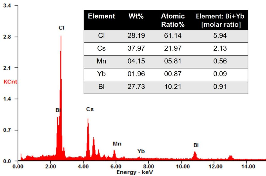
**Figure S6.** Energy Dispersive X-Ray Spectroscopy (EDS) of 10% Yb doped  $\text{Cs}_4\text{MnBi}_2\text{Cl}_{12}$  powder.
