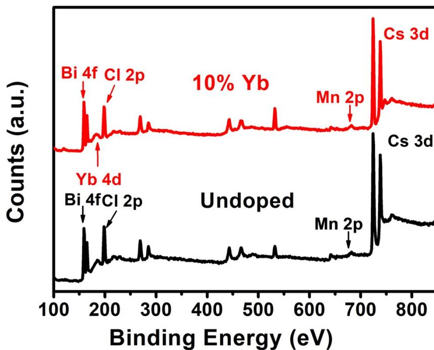
**Figure S4.** The XPS (X-ray photoelectron spectroscopy) survey spectrum of dosages of 10% Yb doped and undoped  $\text{Cs}_4\text{MnBi}_2\text{Cl}_{12}$  powder. The high-resolution XPS spectrum of a) Cs 3d, b) Mn 2p, c) Bi 4f, d) C 1s, e) Cl 2p and f) Yb 4d.
