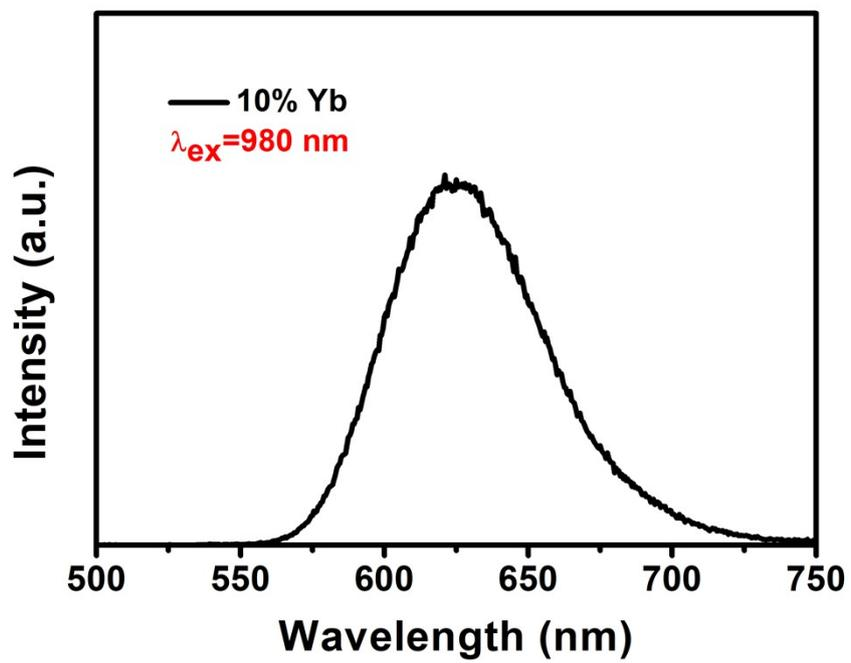
**Figure S12.** The PL spectra of the prepared 10% Yb<sup>3+</sup> doped Cs<sub>4</sub>MnBi<sub>2</sub>Cl<sub>12</sub> powder sample. The results are excited by the 980 nm diode laser with the power from 180 mW to 1190 mW.
