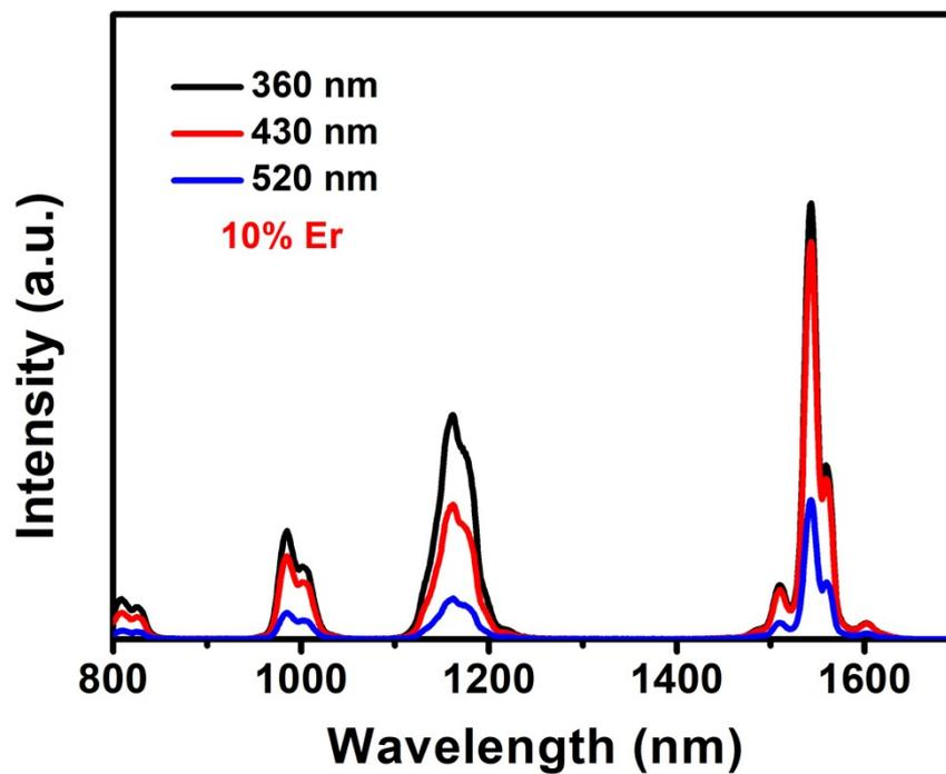
**Figure S17.** The PL spectra of the prepared  $\text{Cs}_4\text{MnBi}_2\text{Cl}_{12}$  samples co-doped with  $\text{Yb}^{3+}$ - $\text{Er}^{3+}$  ions. Excited by the 360 nm laser at 300K.
