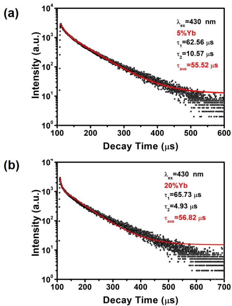
**Figure S8.** PL decay dynamics at 300 K for emission at 580 nm arising from dosages of 5% a) and 20% b)  $\text{Yb}^{3+}$  doped  $\text{Cs}_4\text{MnBi}_2\text{Cl}_{12}$ . Excitation was at 520 nm.
