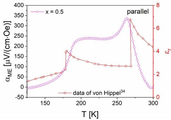
**Figure S8:** Temperature dependence of the magnetoelectric coefficient of the  $\text{Co}_{0.5}/(\text{BaTiO}_3)_{0.5}$  composite in comparison with the dielectric constant of  $\text{BaTiO}_3$  (according von Hippel<sup>34</sup>).
