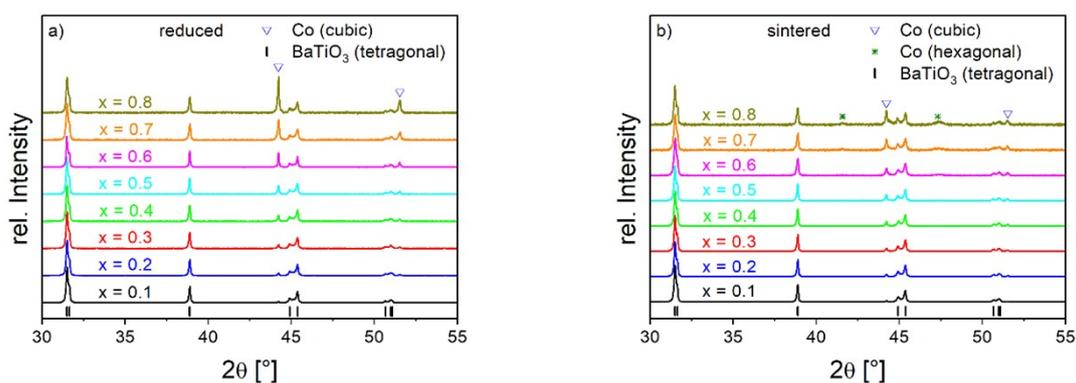
**Figure S1:** XRD patterns of all Co<sub>x</sub>/(BaTiO<sub>3</sub>)<sub>1-x</sub> composites after reduction in forming gas at 1073 K for 2 h (a) and after sintering in nitrogen at 1623 K for 2 h with carbon as oxygen getter (b).
