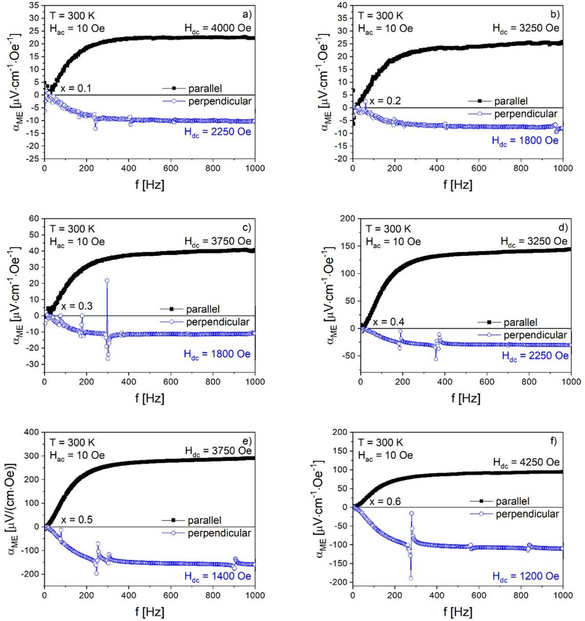
**Figure S7:** Influence of the frequency of the magnetic AC-field on  $\alpha_{ME}$  for  $\text{Co}_x/(\text{BaTiO}_3)_{1-x}$  samples with  $x = 0.1$  (a),  $0.2$  (b),  $0.3$  (c),  $0.4$  (d),  $0.5$  (e) and  $0.6$  (f) in parallel (black filled squares) and perpendicular orientation (blue open squares).
