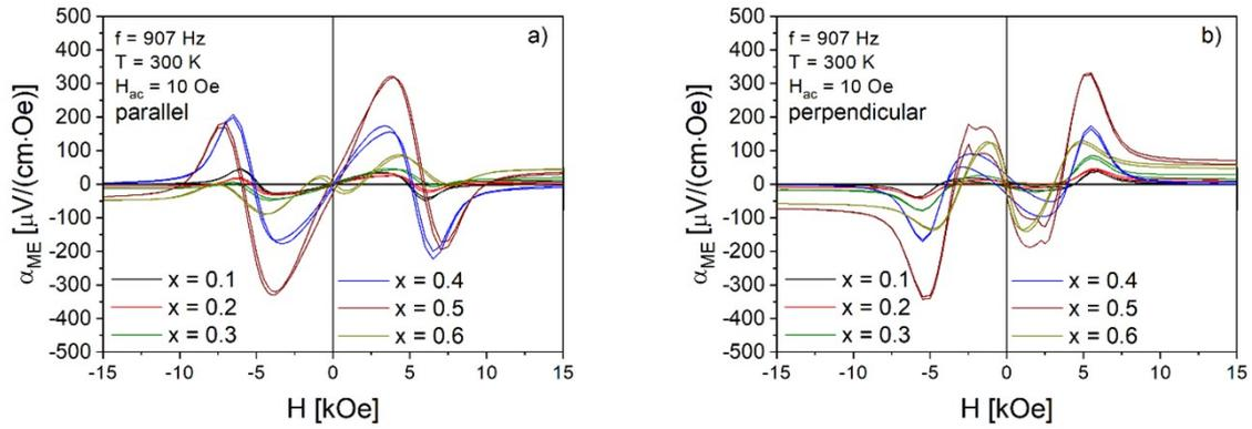
**Figure S6:** Field dependence of the magnetoelectric coefficients of the  $\text{Co}_x/(\text{BaTiO}_3)_{1-x}$  samples ( $x = 0.1$  to  $0.6$ ) for parallel (a) and perpendicular orientation (b).
