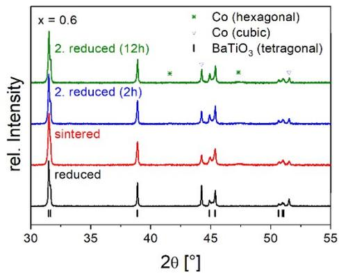
**Figure S3:** XRD patterns of  $\text{Co}_{0.6}/(\text{BaTiO}_3)_{0.4}$  after reducing in forming gas at 1073 K for 2 h, sintering in nitrogen at 1623 K for 2 h with carbon as oxygen getter and after a further reductive sintering in forming gas at 1073 K for 2 or 12 h.
