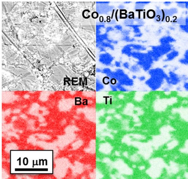
**Figure S4:** REM and EDX area scan of  $\text{Co}_{0.8}/(\text{BaTiO}_3)_{0.2}$ .
