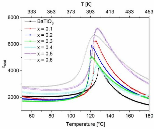
**Figure S5:** Temperature dependence of the relative permittivity of  $\text{Co}_x/(\text{BaTiO}_3)_{1-x}$  with  $x = 0.1$  to  $0.6$  measured at  $1 \text{ kHz}$ .
