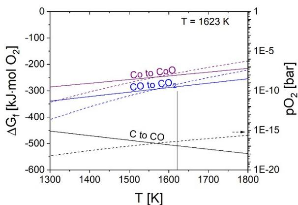
**Figure S2:** Calculated standard Gibbs free energies of oxide formation for cobalt and carbon (full lines), based on data from Barin et al.<sup>48</sup> and the corresponding equilibrium oxygen pressures (dashed lines).
