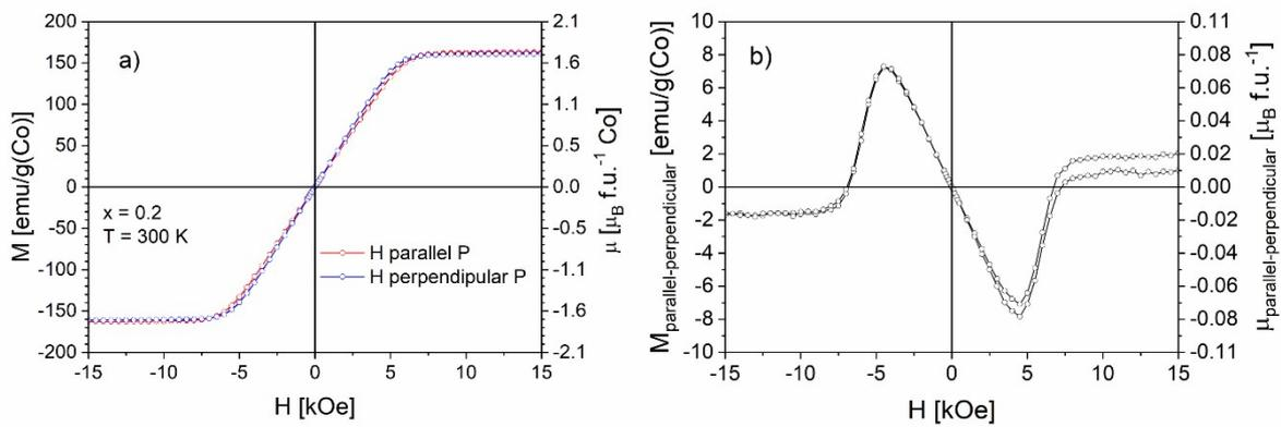
**Figure S9:** Comparison of  $M$  vs.  $H$  for an  $P\parallel H$  and  $P\perp H$  electrically poled  $\text{Co}_{0.2}/(\text{BaTiO}_3)_{0.8}$  composite (a) and the difference between the observed magnetizations as a function of the magnetic field (b).
