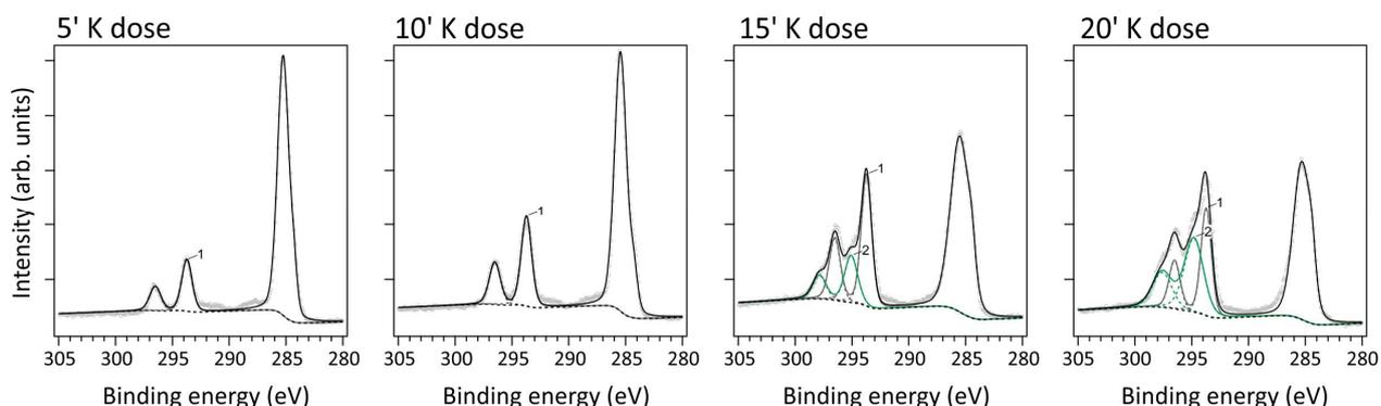
**Figure S1.** K 2p and C 1s XPS spectra acquired at the NiTPP/Au(111) interface as a function of the potassium evaporation time.
