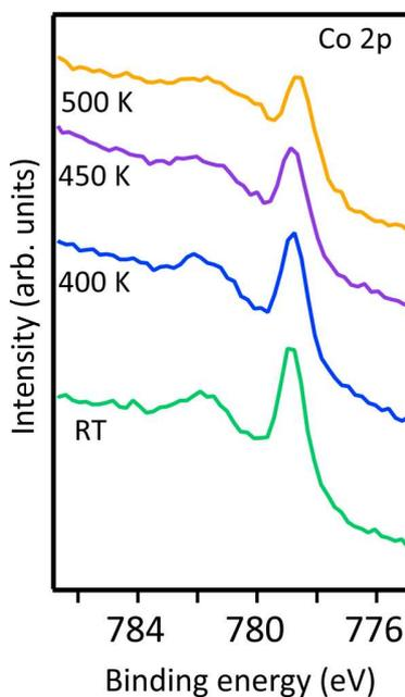
**Figure S4.** Co  $2p_{3/2}$  core level of CoTPP/Au(111) after exposure to K for 15 minutes at room temperature (green curve) and for increasing annealing temperatures.
