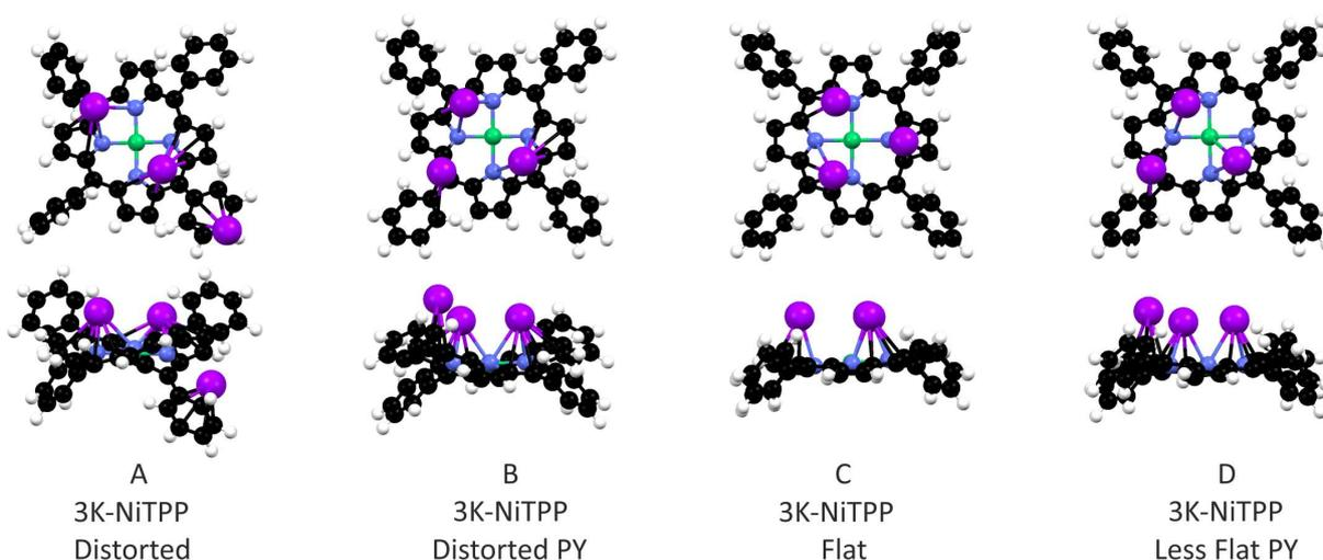
**Figure S3.** A schematic representation of the different K adsorption geometries calculated for the 3K-NiTPP complex. Black, white, blue, green, and violet spheres represent C, H, N, Ni, and K, respectively.
