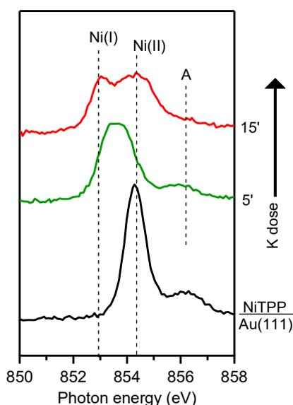
**Figure S2.** Ni L<sub>3</sub>-edge NEXAFS spectrum acquired in s-polarization for the pristine NiTPP/Au(111) interface and after exposure to increasing K doses (5 and 15 minutes dose).
