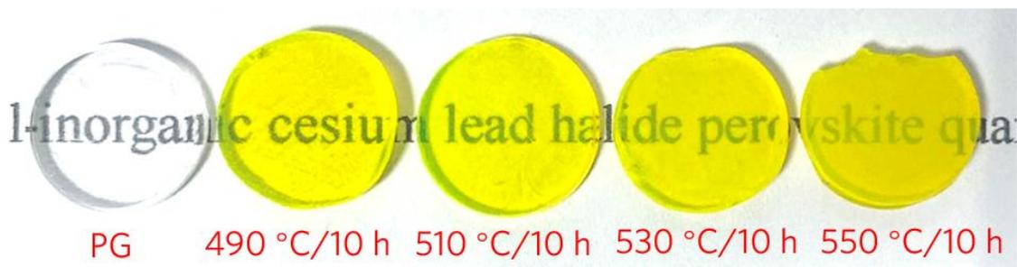
**Fig. S3.** Photographs of CsPbBr<sub>3</sub> QDs@glass specimens of GC-CaF<sub>2</sub> after heat treatment at different temperatures for 10 h.
