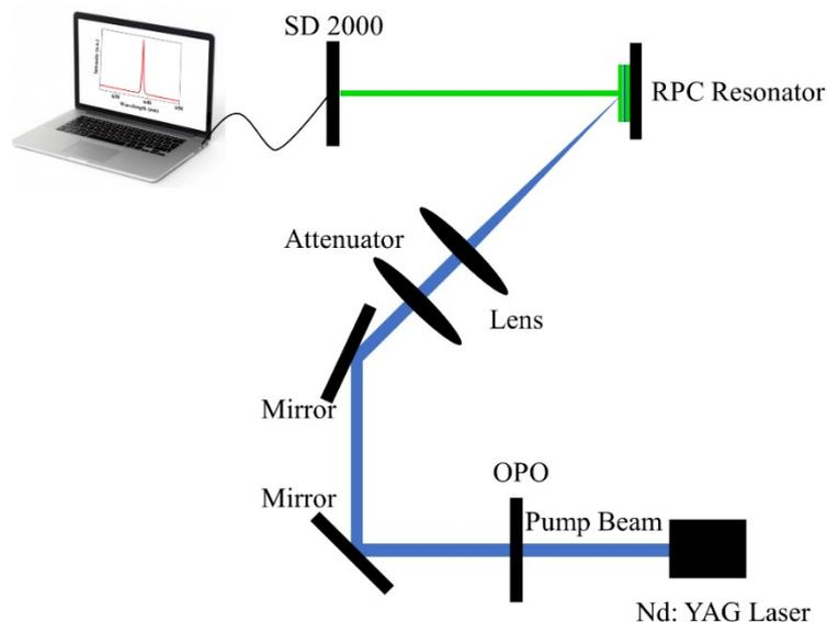
**Figure S17.** Schematic diagram of the home-made measurement equipment for the emission spectra under the pulsed Nd: YAG laser irradiation
