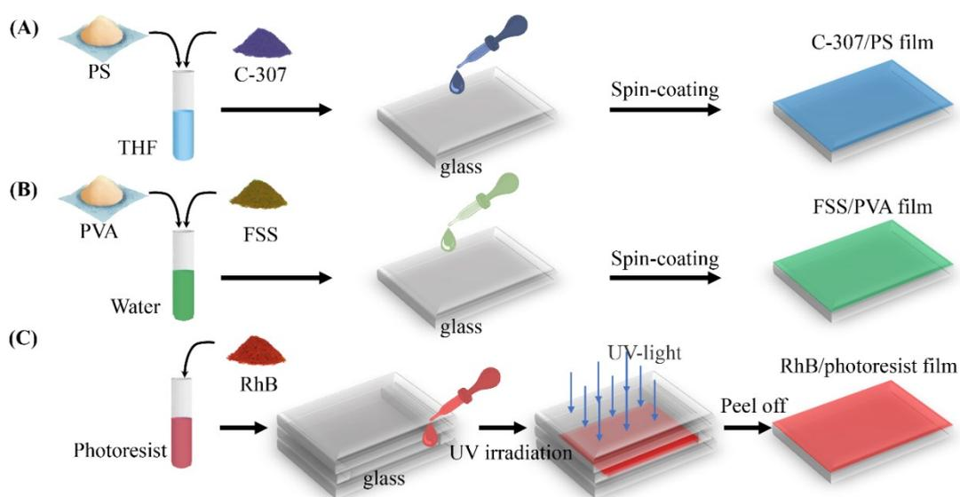
**Figure S7.** Schematic diagram of the preparation of dye doped polymer films with different colors. The process of fabricating (A) C-307/PS film, (B) FSS/PVA film, and (C) RhB/photoresist film
