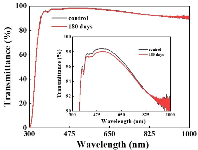
**Fig. S1** 95.1% of the transmittance is for the AHMA/Glass (control), and 94.9% after 180 days under light illumination.
