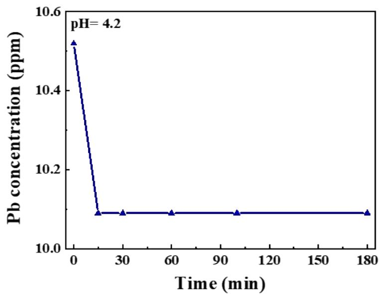
**Fig. S3** Lead ion concentration tracking of  $\text{PbNO}_3$  solution (pH= 4.2) soaked with AHMA film at 40 °C (140 mg of AHMA coated on 25\*25mm of glass).
