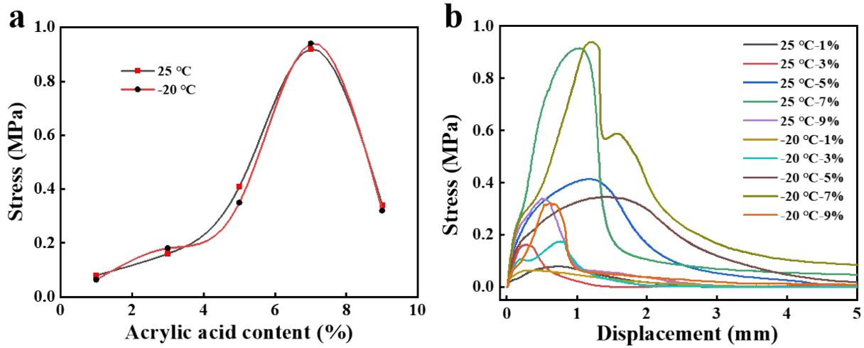
**Fig. S6** Good cold resistance of the AHMA materials has been confirmed, the bond shear strength of which at -20 °C is consistent with that at room temperature.
