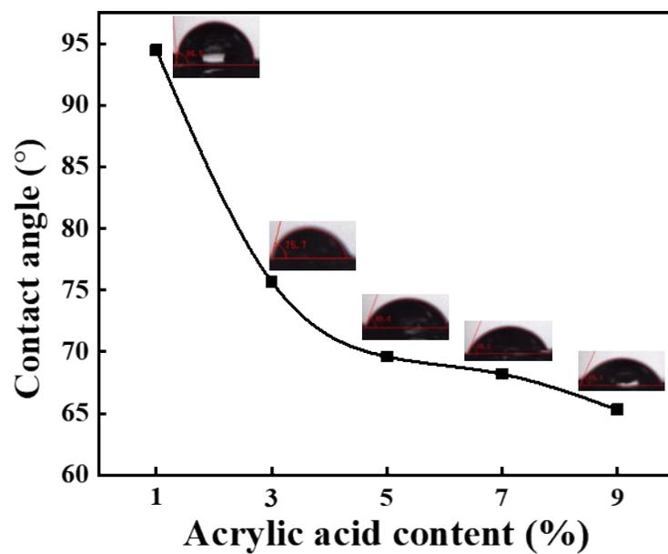
**Fig. S2** The water contact angle of AHMA with different acrylic acid content.
