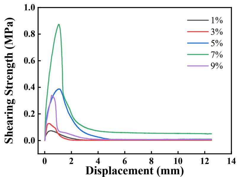
**Fig. S4** Shear strength between glass and AHMA with different content of acrylic acid. Two glasses sheets bonded by a AHMA film (12.5 mm \* 25 mm). It was measured on an electronic universal testing machine at a deflection rate of 5 mm/min.
