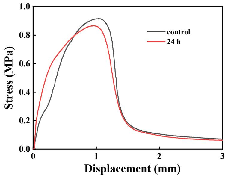
**Fig. S11** After soaking in water for 24 hours, the bonding shear strength between AHMA with 7% of acrylic acid and glass decreased by less than 0.05 MPa.
