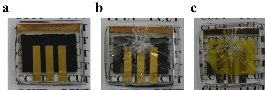
**Fig. S8** Lead leakage on perovskite modules. (a) Image of the PSCs encapsulated with PVB-glass. (b) Images of the damaged PSCs encapsulated with PVB-glass by falling ball impact with a 100 g of steel ball at 50.8 cm of high. (c) Images of the damaged PSCs after dripping by heavy rainfall (pH=4.2) at 5 mL h<sup>-1</sup> for 6 h.
