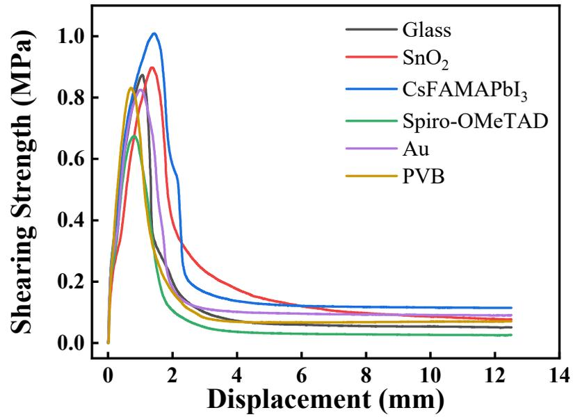
**Fig. S7** The shear strengths among AHMA with different materials of each layer in photovoltaic building integrated module.
