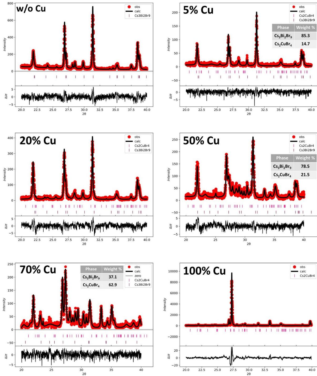
Fig. S4 Rietveld refinement spectra of different Cu-alloyed perovskite thin films.
