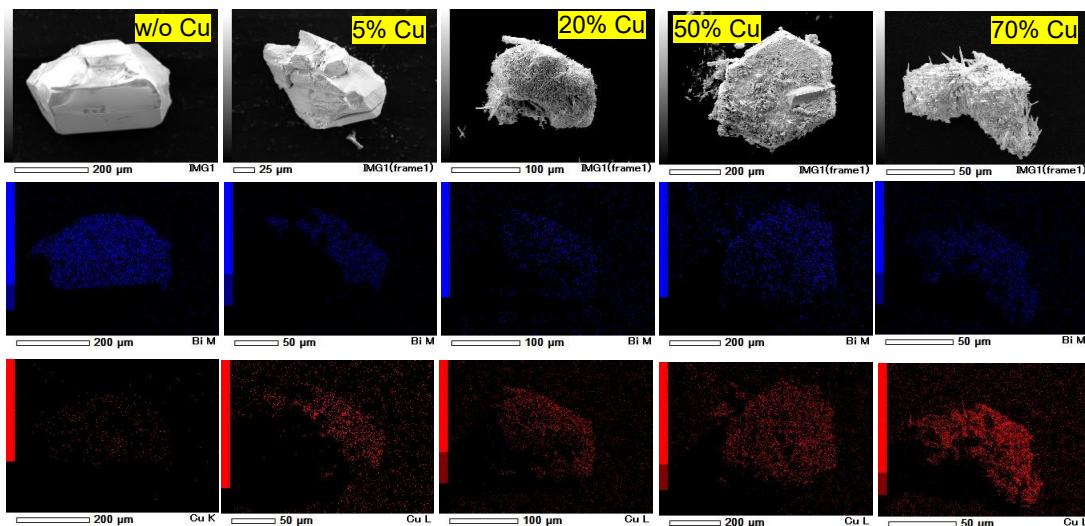
**Fig. S1** Scanning Electron Microscope (SEM) images of perovskite crystals with different Cu-alloying with Energy Dispersive Scanning (EDS) elemental mapping for Bi (Blue) and Cu (Red).
