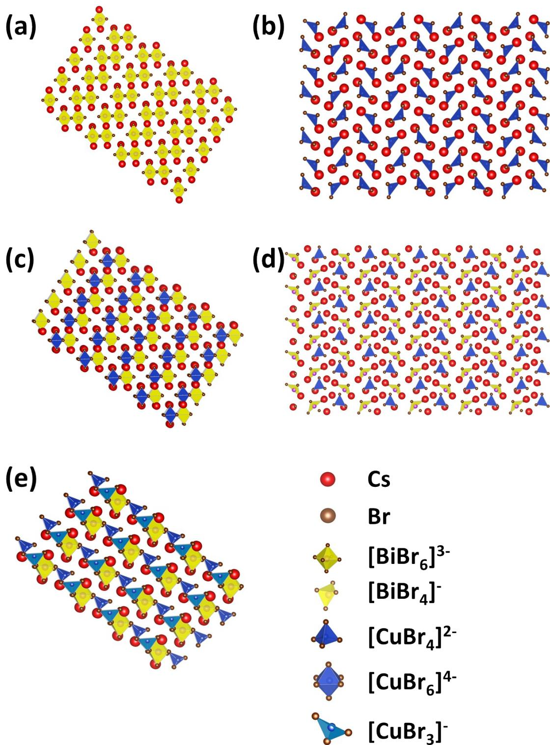
**Fig. S10** Different perovskite crystal structures applied for calculating energy above the convex hull: (a)  $\text{Cs}_3\text{Bi}_2\text{Br}_9$  (b)  $\text{Cs}_2\text{Cu}\text{Br}_4$  (c) 50%Cu- $\text{Cs}_3\text{Bi}_2\text{Br}_9$  (d) 50%Cu- $\text{Cs}_2\text{Cu}\text{Br}_4$  (e)  $\text{Cu}_-\text{Cs}_3\text{Bi}_2\text{Br}_9 \text{ CuBr}$  compensating defect.
