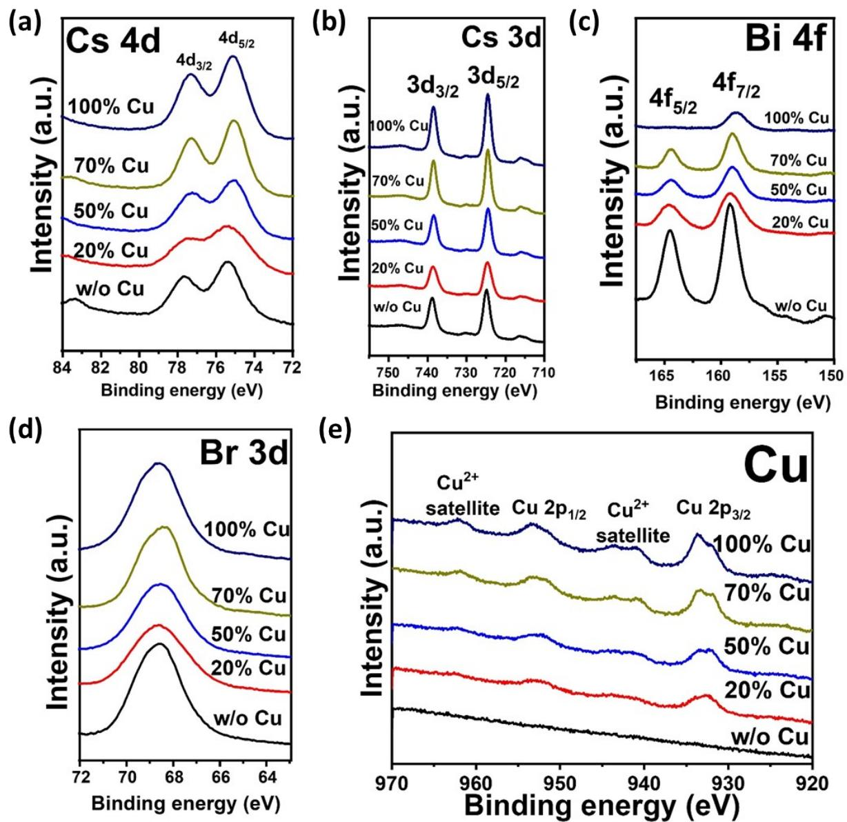
Fig. S9 XPS spectra of Cs 4d (a), Cs 3d (b), Bi 4f (c), Br 3d (d), and Cu 2p (e) for different alloyed Cu-Cs<sub>3</sub>Bi<sub>2</sub>Br<sub>9</sub> perovskites.
