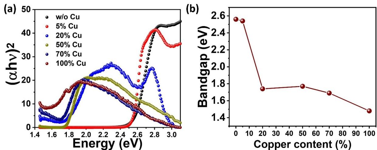
Fig. S3 Direct bandgap estimation: (a) Tauc plots of different Cu-alloyed perovskite thin films. (b) Bandgap energies of different Cu-alloyed perovskite thin films.
