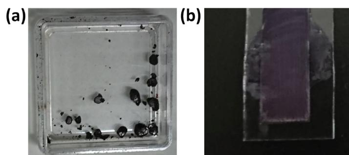
**Fig. S2** (a) Photograph of  $\text{Cs}_2\text{CuBr}_4$  perovskite crystals. (b) Photograph of drop-casted  $\text{Cs}_2\text{CuBr}_4$  perovskite thin film over  $\text{TiO}_2/\text{Glass}$  substrate.
