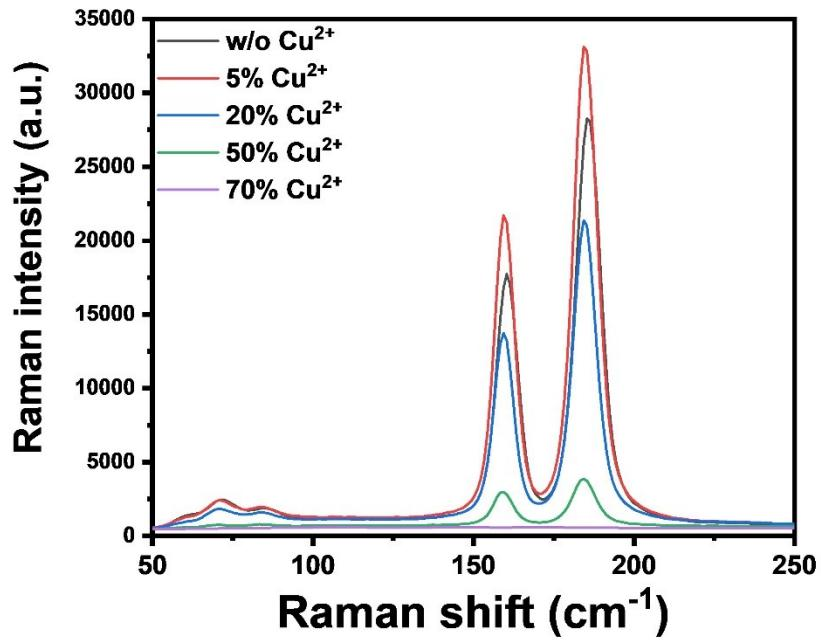
**Fig. S6** Raman measurement of different Cu-alloyed perovskite crystals.
