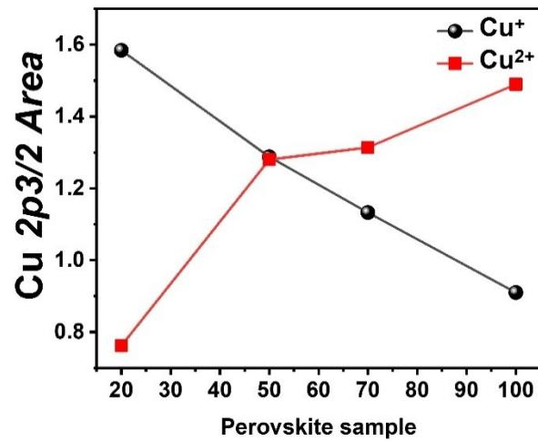
Fig. S8 XPS Cu 2p<sub>3/2</sub> peak area of Cu<sup>2+</sup> (Red square) and Cu<sup>+</sup> (Black balls) for different alloyed Cu- $\text{Cs}_3\text{Bi}_2\text{Br}_9$  perovskites.
