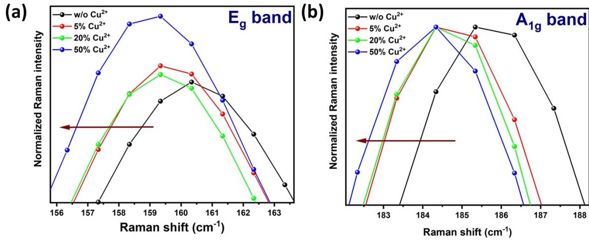
Fig. S7 Normalized Raman Eg (a), and A1g (b) bands for different alloyed Cu- $\text{Cs}_3\text{Bi}_2\text{Br}_9$  perovskites.
