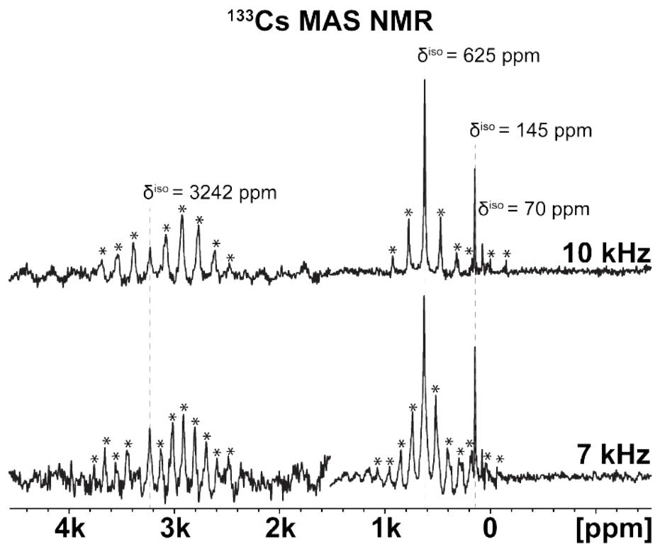
**Fig. S5** Experimental  $^{133}\text{Cs}$  MAS NMR spectra of 70% Cu-alloyed perovskite were conducted at 10 kHz and 7 kHz spinning speeds of the sample. The asterisks (\*) denote spinning sidebands.
