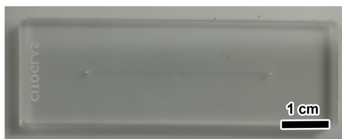
Fig. S4 Digital image of the microfluidic chip used in the experiment.
