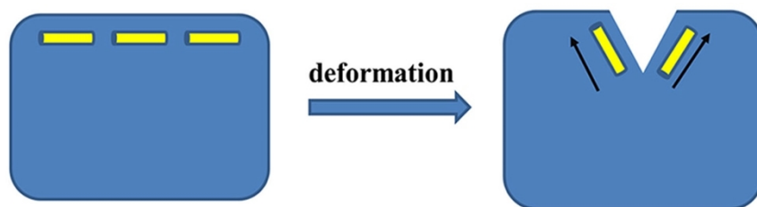
Fig. S15 Schematic diagram of the moving process of the nanorods in the film caused by the liquid flow generated from the deformation.
