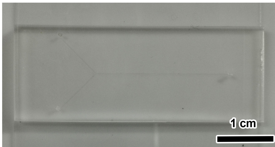
Fig. S17 Digital photo of the microfluidic chip used in the experiment. The suspension was flowing from the right entrance to the left branched exit. The exit was blocked or circulated.
