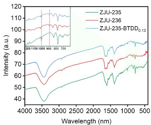
**Figure S8.** FT-IR spectra of ZJU-235, ZJU-236 and ZJU-235-BTDD<sub>0.13</sub>.
