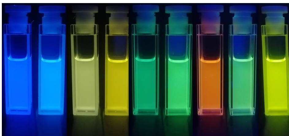
Fig. S6 Photographs of 3a–3i taken under UV light (365 nm) in DCM.
