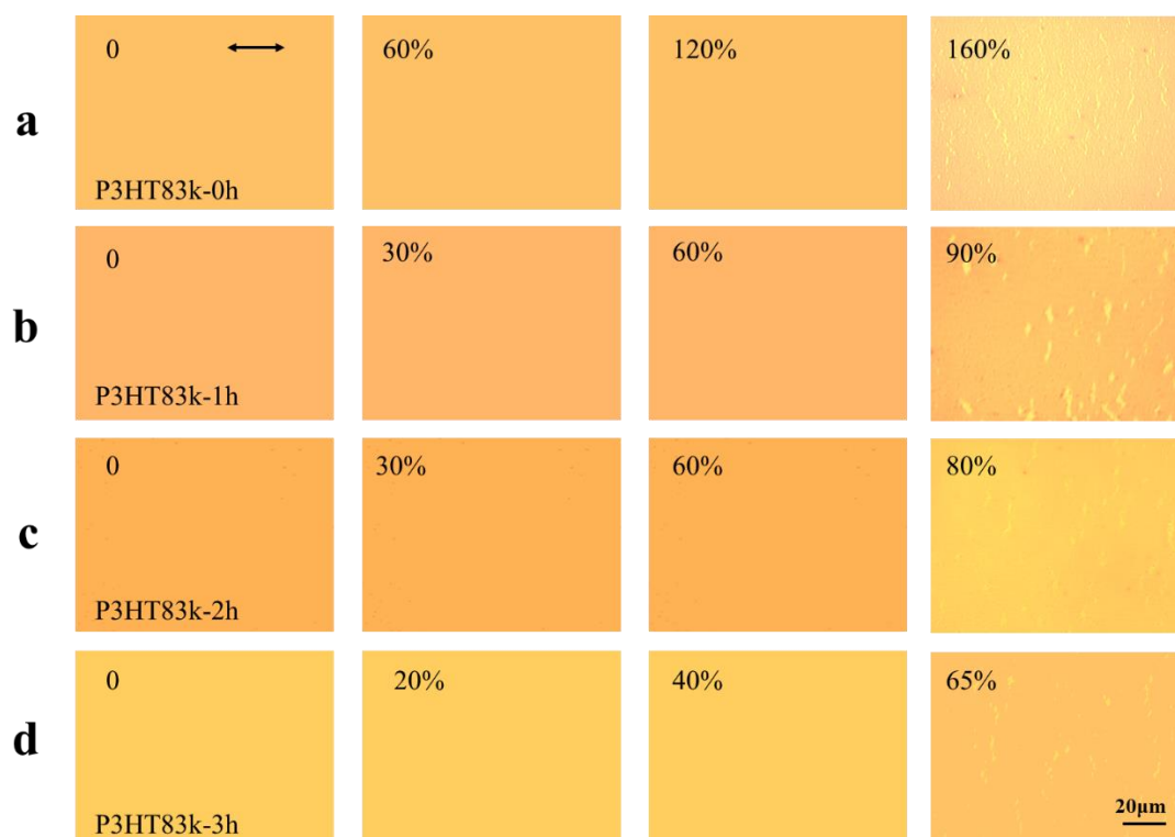
Figure S5. Optical microscopy images of P3HT83k films elongated under different strains. The samples were annealed by ODCB vapor for different time: (a) 0 h, (b) 1 h, (c) 2 h and (d) 3 h.
