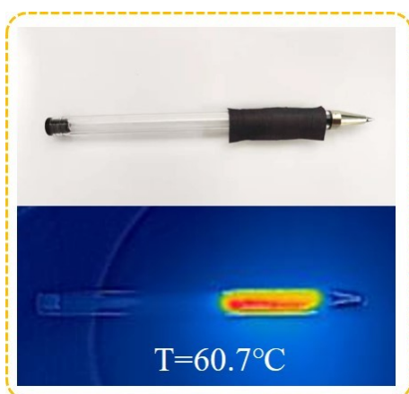
Fig. S37. Photographs of AgNPs 6 @MNWF 5 wrapped on a pen and the corresponding IR image.
