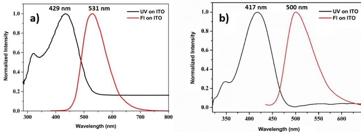
Figure S1. Absorbance and emission of a) M1 and b) M2 on ITO
