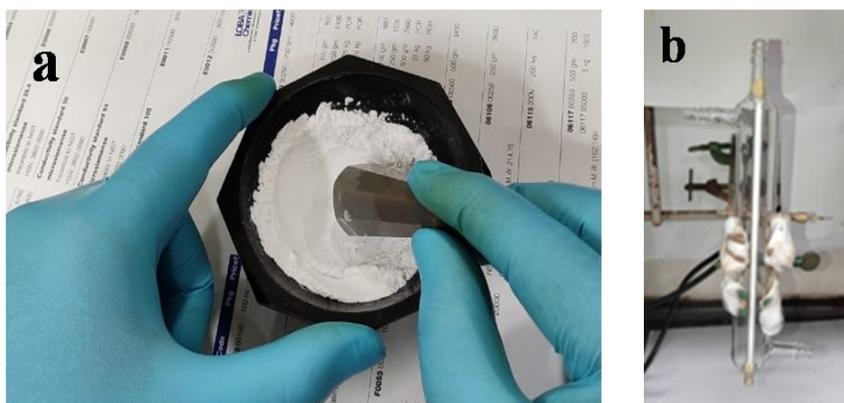
a) Homogeneous mixture of  $K_2CO_3$  and Celite, and b) packed glass column reactor with  $K_2CO_3$  and celite
