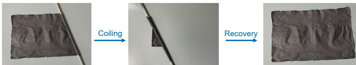
Fig. S17. Coiling demonstration of as-prepared \text{Ti}_3\text{C}_2\text{T}_x/\text{MLPAN} hybrid fabric.
