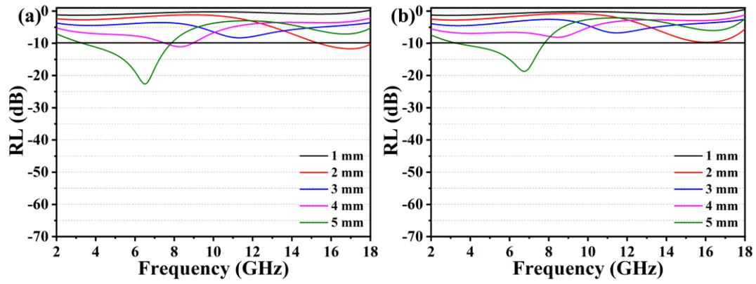
**Fig. S3** Reflection loss versus frequency plot of (a)  $\text{Fe}_3\text{O}_4$ , (b)  $\text{Fe}_3\text{O}_4@\text{mSiO}_2$  in the frequency range of 2-18 GHz.
