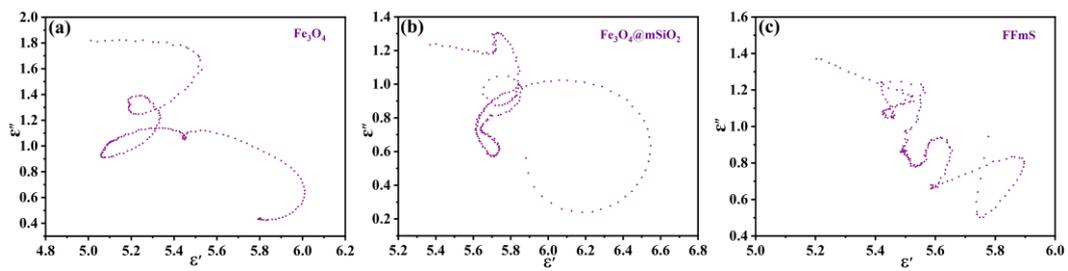
**Fig. S2** The  $\epsilon''$  versus  $\epsilon'$  of (a)  $Fe_3O_4$ , (b)  $Fe_3O_4@mSiO_2$  and (c) FFmS.
