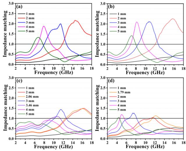
**Fig. S5** Impedance matching of  $\text{Fe}_3\text{O}_4$  (a),  $\text{Fe}_3\text{O}_4@\text{mSiO}_2$  (b), FFmS (c) and FFmSR (d) with different thicknesses.
