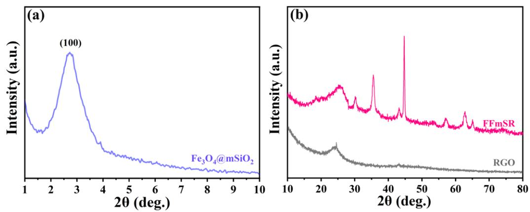
**Fig. S1** (a) low-angle XRD patterns of  $\text{Fe}_3\text{O}_4@m\text{SiO}_2$ . (b) XRD patterns RGO and FFmSR.
