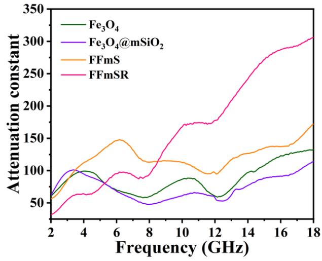
**Fig. S4** Frequency-dependent attenuation constant of Fe<sub>3</sub>O<sub>4</sub>, Fe<sub>3</sub>O<sub>4</sub>@mSiO<sub>2</sub>, FFmS and FFmSR.
