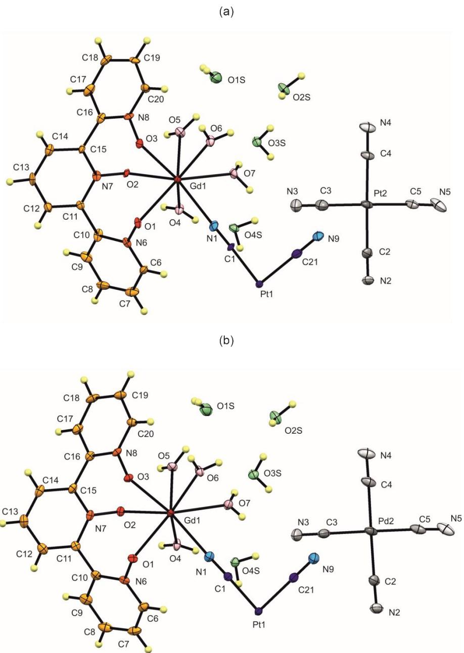
**Fig. S8** Asymmetric units of **Gd<sub>2</sub>Pt<sub>3</sub>** (a) and **Gd<sub>2</sub>Pd<sub>3</sub>** (b) with the atoms labeling schemes. Thermal ellipsoids are presented at the 50% probability level. The related bond lengths and angles are collected in Tables S11 and S12.
