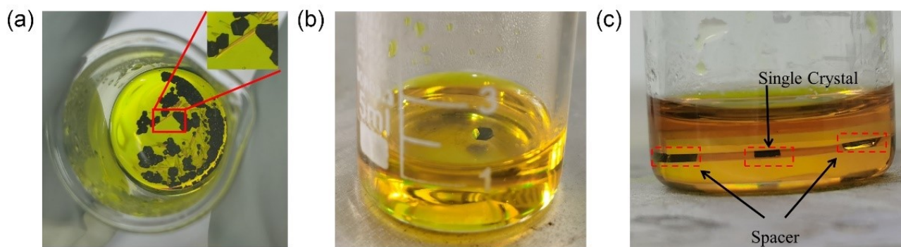
Fig. S3 Grow FAPbI 3 SC a) without using the seeds, the inset shows needle-like yellow \delta -FAPbI 3 perovskites. b) using the seeds. c) using the SCITC method.
