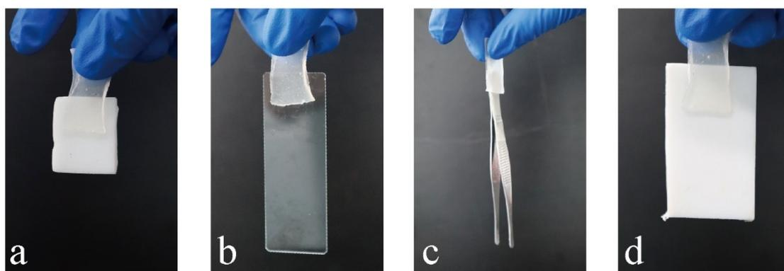
**Figure S5.** The hydrogel exhibits an excellent adhesion property by adhering to (a) general silicon rubber (TT630, Shenzhen Hong Ye Jie Technology Co., Ltd, Shenzhen, China; ~3.1 g), (b) glass slide (~5.02 g), (c) metal tweezer (~15.6 g), and (d) poly tetra fluoroethylene (PTFE) sheet (~22.2 g) with the contact area of ~ 1.0 cm<sup>2</sup>.
