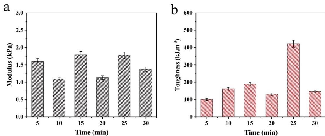
**Figure S3.** The modulus (a) and toughness (b) of PVA-CS-PAM hydrogels as function of soaking time in borax solution.
