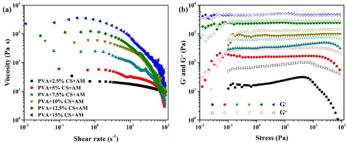
**Figure S1.** (a) The shear-thinning behavior and (b) the storage modulus ( $G'$ ) and loss modulus ( $G''$ ) of the PVA-CS-AM hydrogel ink with different concentrations of CS.
