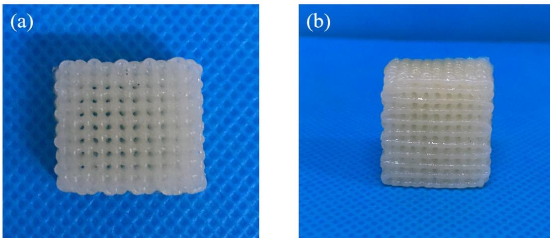
**Figure S6.** The 3D printed hydrogel cellular structure photos from (a) top and (b) front view.
