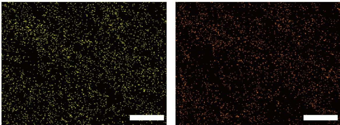
**Figure S2.** Na (left) and B (right) elements on the surface of freeze-dried ionic conductive hydrogel (scale bar is 50  $\mu m$ ).
