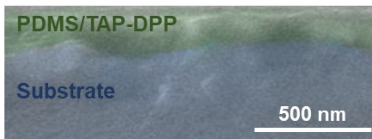
Fig. S11 Cross-sectional SEM image of PDMS/TAP-DPP film after continuous operation for 200,000 cycles.
