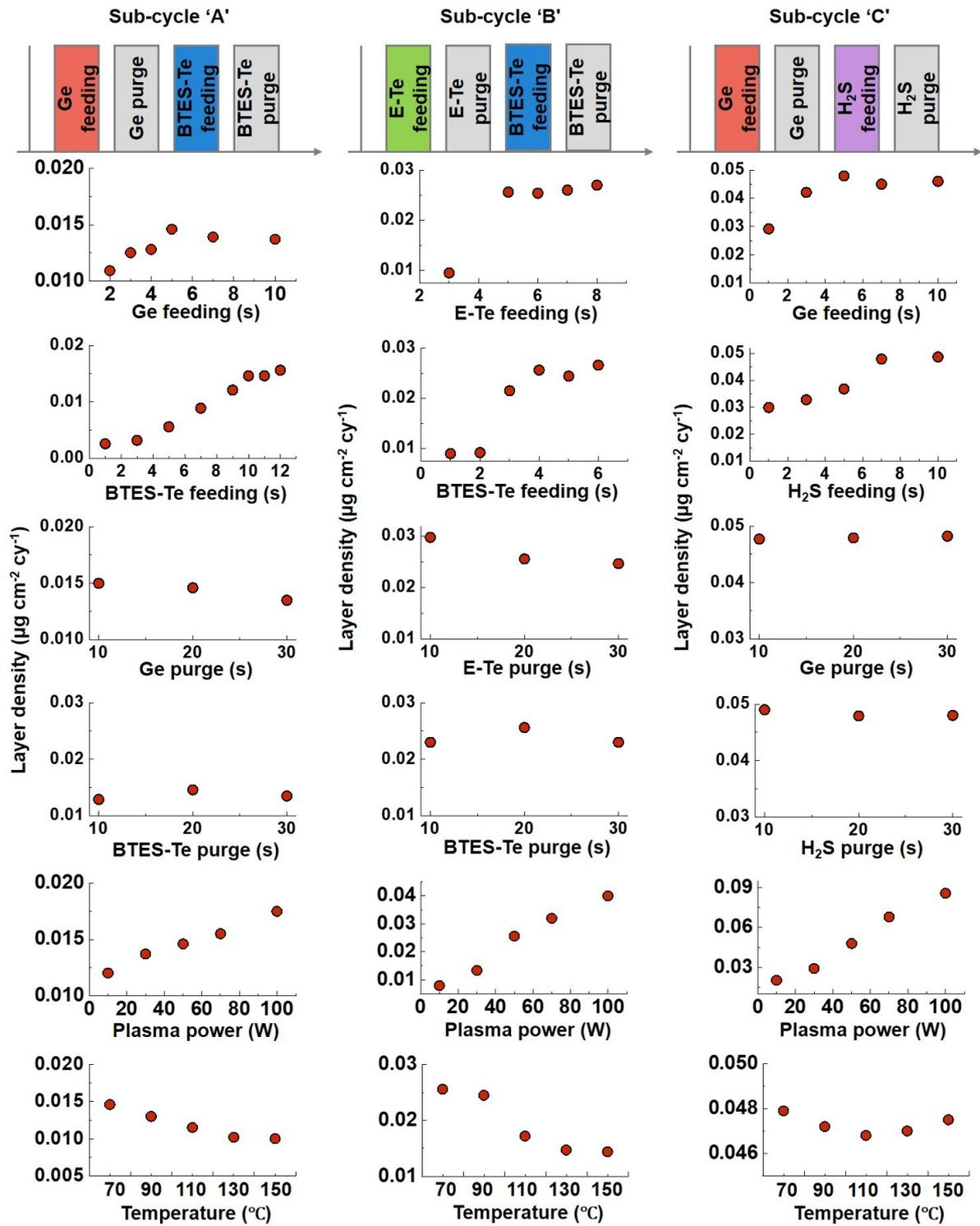
**Figure S1.** From the left to the right vertical panel, the detailed ALD process developments of Ge-Te, Te-Te, and Ge-S sub-cycles are shown. In each ALD process development, the ALD
