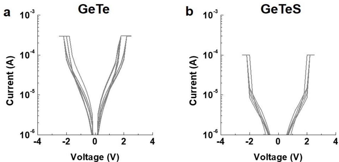
**Figure S4.** a and b show the DC I-V curves of 10 cycles of the GT- and GTS-based TS devices.
