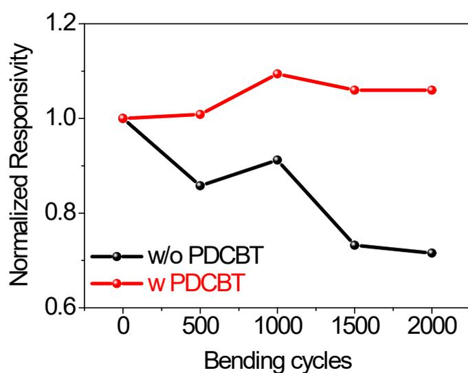
**Figure S4.** Normalized responsivity of MAPbI<sub>3-x</sub>Cl<sub>x</sub>-based FSPPD as a function of
