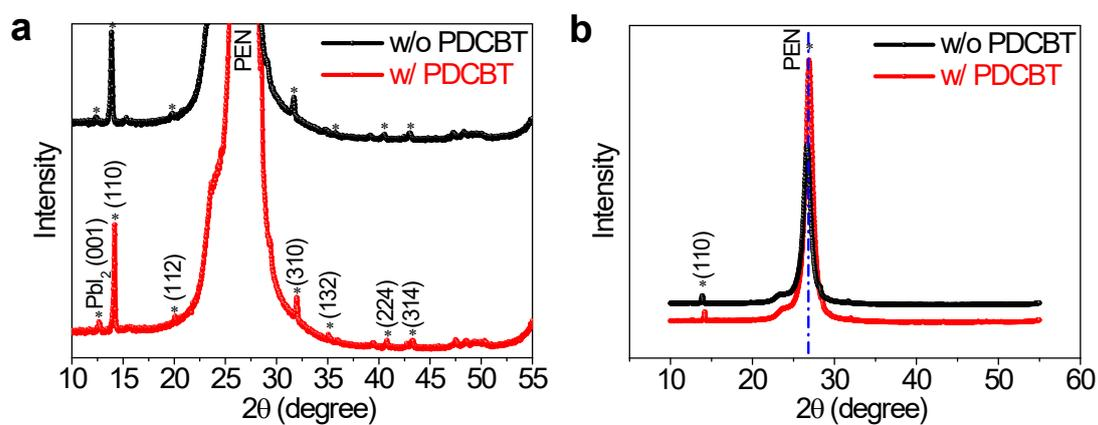
**Figure S6.** XRD patterns of MAPbI<sub>3-x</sub>Cl<sub>x</sub> film prepared with/without PDCBT (a) excluding and (b) including PEN peak.
