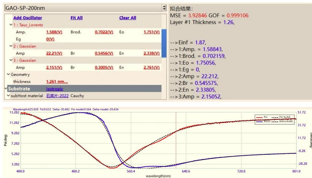
**Figure S1.** The thicknesses of PDCBT layer, which was measured by an ellipsometer.
