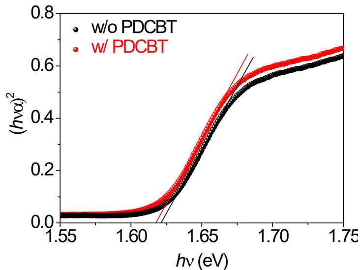
**Figure S9.** The band edges of  $\text{MAPbI}_{3-x}\text{Cl}_x$  film prepared with/without PDCBT determined from Tauc plots.
