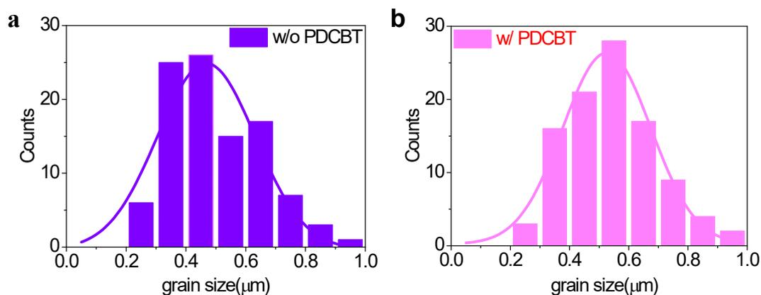
**Figure S5.** Grain size distribution histogram of MAPbI<sub>3-x</sub>Cl<sub>x</sub> film prepared (a) without PDCBT and (b) with PDCBT, obtained by the top view of SEM images.
