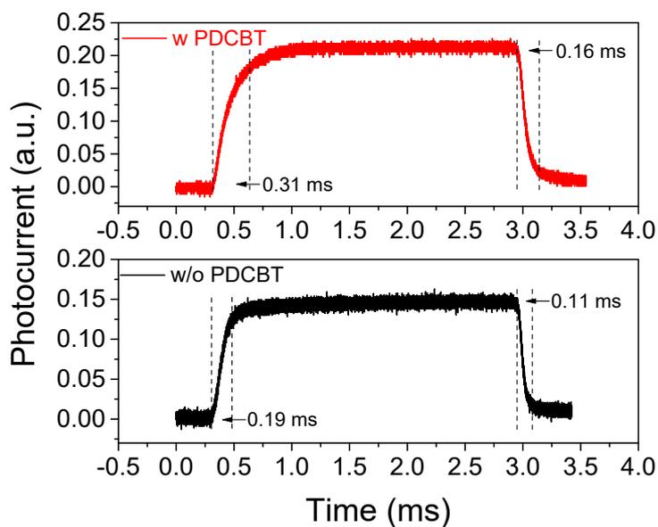
**Figure S3.** The rise time/decay time for FSPPD with/without PDCBT layer. The rise time of FSPPD was calculated by the time interval for the photocurrent to reach 90% of its highest value, while the decay time was calculated by the time interval for the photocurrent to fall 10% of its highest value.
