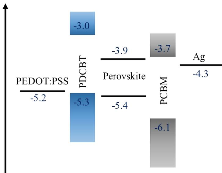
**Figure S10.** Energy level diagram of the FSPPD with PDCBT.
