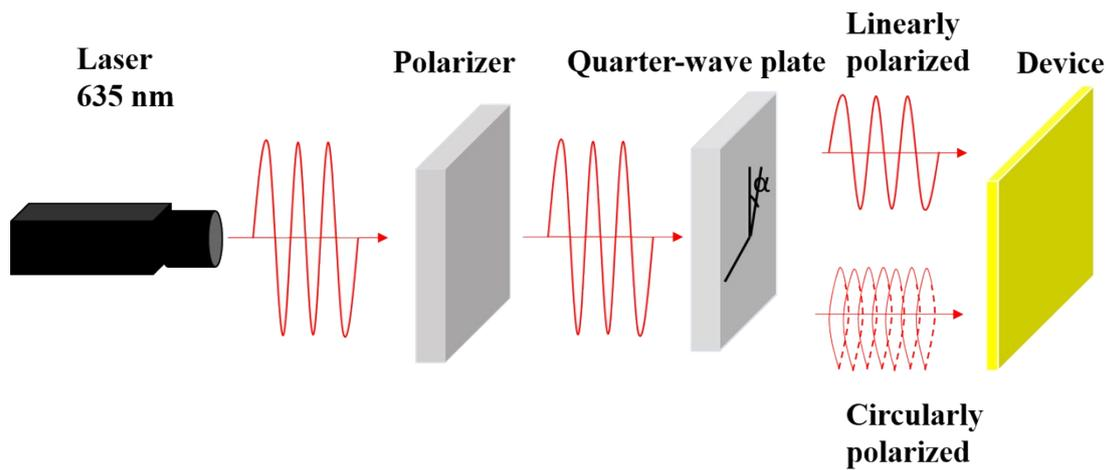
**Figure S7.** Experimental setup for the linear/circular photoexcitation-modulated photocurrent measurements.
