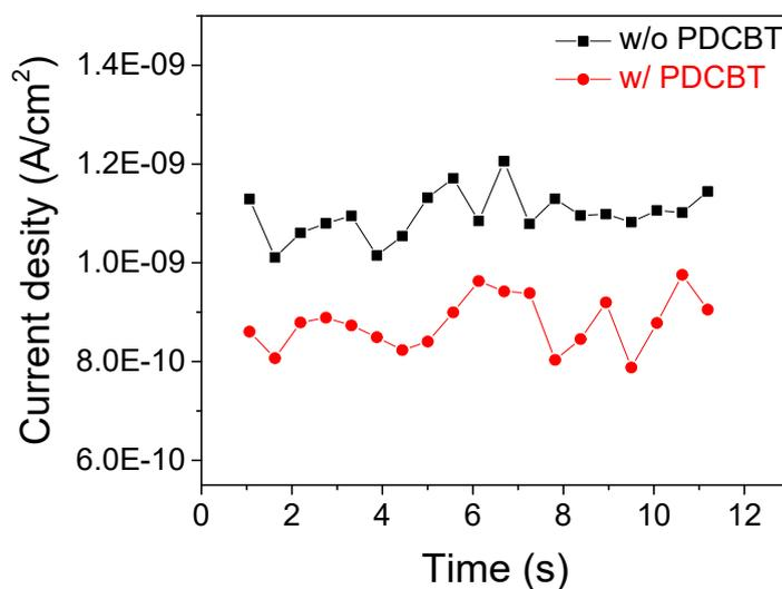
**Figure S2.** Dark current density under zero bias of MAPbI<sub>3-x</sub>Cl<sub>x</sub>-based FSPPD
