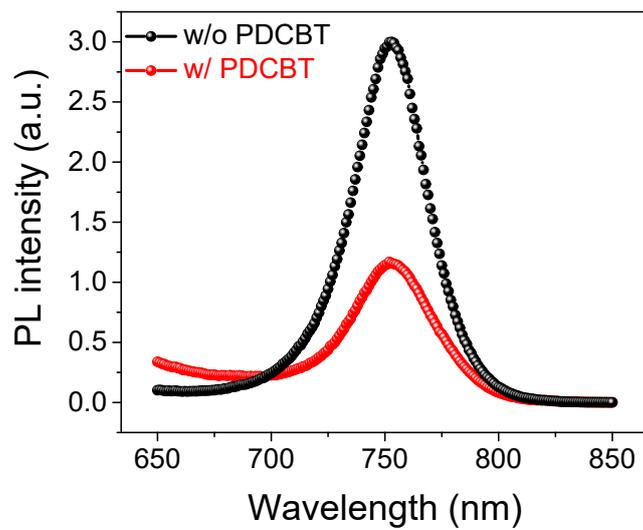
**Figure S8.** PL spectra of MAPbI<sub>3-x</sub>Cl<sub>x</sub> films prepared with/without PDCBT.
