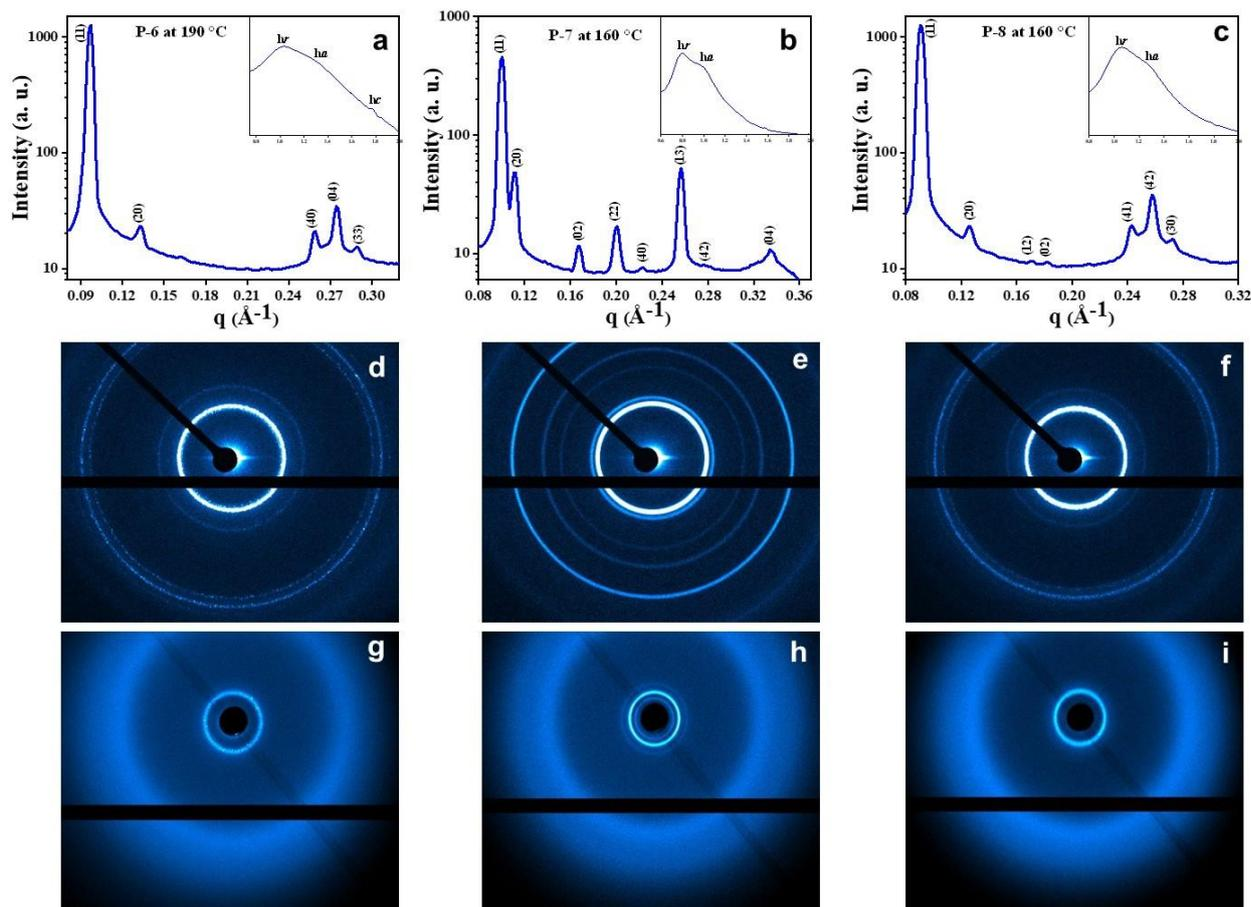
**Fig. S18** Small and wide angle (inset) X-ray diffraction patterns of compound (a) **P-6** at 190 °C ( $\text{Col}_r$ ), (b) **P-7** at 160 °C ( $\text{Col}_r$ ) and (c) **P-8** at 160 °C ( $\text{Col}_{ob}$ ) upon cooling,  $h_r$  - cholesterl-cholesterol correlation,  $h_a$  - alkyl chain-chain correlation. The lower panel shows the respective 2D diffraction patterns of SAXS (d, e, f) and WAXS (g, h, i).
