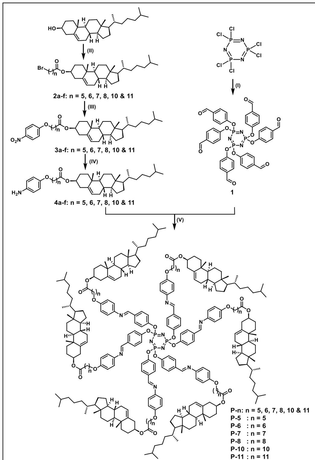
**Reagents and conditions:** (I) 4-Hydroxybenzaldehyde,  $\text{K}_2\text{CO}_3$ , THF,  $70^\circ\text{C}$ , 48 h, 60 %; (II) DCC, DMAP, dry DCM,  $60^\circ\text{C}$ , 12 h, (Yield = 75 - 78 %); (III) 4-nitrophenol,  $\text{K}_2\text{CO}_3$ , butanone, KI,  $90^\circ\text{C}$ , 24 h, (Yield = 85 - 90 %); (IV)  $\text{H}_2$ , 10 % Pd/C, THF, RT, 48 h, (Quantitative Yield); (V) dry THF,  $60^\circ\text{C}$ , 24 h (Yield = 35 - 40 %).
