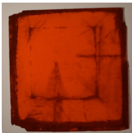
Figure S4. The photograph of the polished crystal. The edge of the inner seed crystal shows a black outline in the figure.
