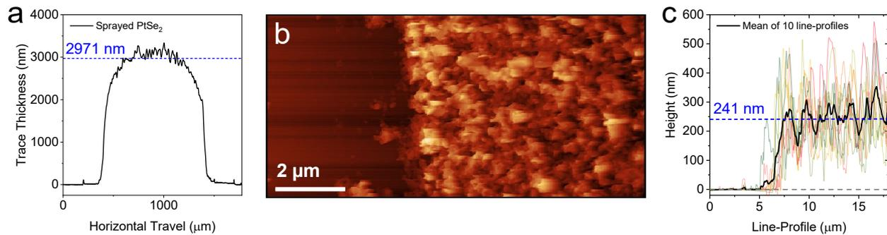
Fig. S2 (a) Profilometry curve indicates  $\sim 3 \mu\text{m}$  of film thickness produced by conventional spray deposition. (b) AFM image of an LPE-PtSe<sub>2</sub> film produced by the modified LB method using two subsequent deposition cycles of the 400-30000 g sample and (c)  $\sim 240 \text{ nm}$  film thickness is estimated from the mean of 10 height profiles.
