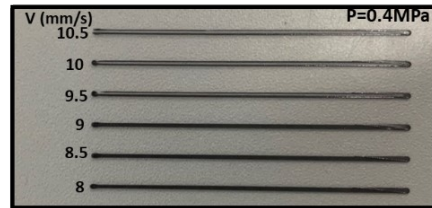
Figure S1. a. Schematic illustration of typical parameters for 3D DIW printing b. The testing printing with different pressure and different velocity.
