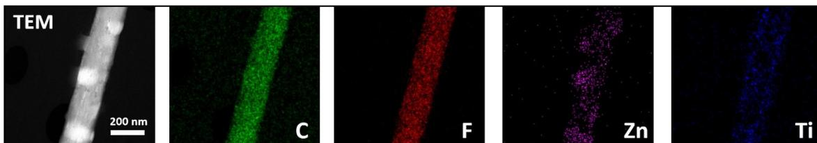
**Fig. S2** TEM and EDS analysis of electrospun MXene-CTAB-ZnO embedded NFs.
