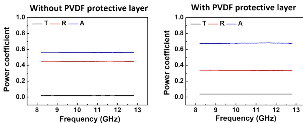
**Fig. S6.** Reflectivity and absorptivity of ZnO NRs decorated PVDF-MXene composite NF. (left) without a protective layer (right) with a protective layer
