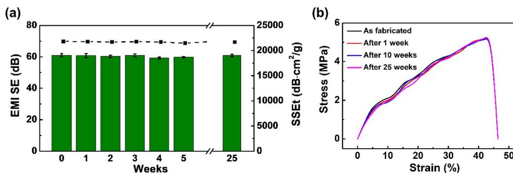
**Fig. S7** Long-term stability of the ZnO NRs decorated PVDF-MXene NFs after 6 months. (a) EMI SE and absolute EMI SE (b) Stress-strain curves.
