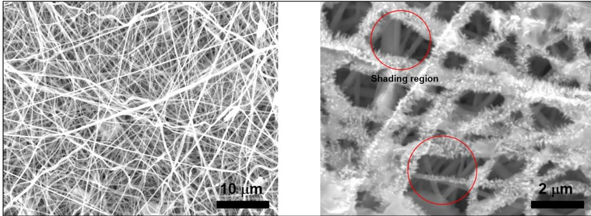
**Fig. S1** SEMs of ZnO NRs decorated PVDF-MXene NFs by sputtering method. Red circles indicate the shaded regions where ZnO seed layer cannot be deposited.
