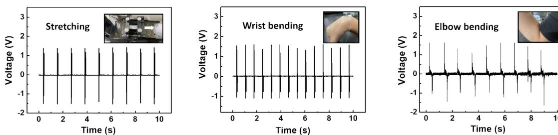
**Fig. S8.** Piezoelectric outputs of ZnO NRs decorated PVDF-MXene NFs based piezoelectric motion sensor under different motions
