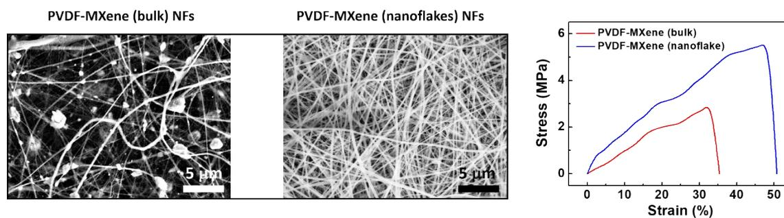
**Fig. S4** (left) SEMs of PVDF-MXene composite NFs containing bulk MXene and MXene nanoflakes (right) stress-strain curves of each NF film
