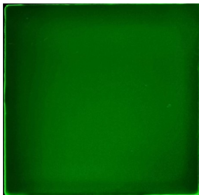
Fig. S6 The digital photograph of Cd 2+ -doped FAPbBr 3 @PVDF (Cd/Pb = 0.7) film, under UV irradiation at 365 nm.
