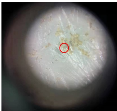
Figure S7. The optical image of \text{CsCu}_2\text{I}_3 micro-rods on the fiber end-facet.
