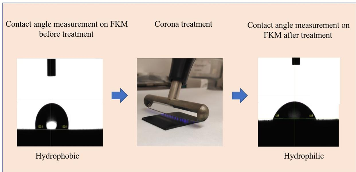
Figure 2. Contact angle measurement on FKM before and after corona treatment.
