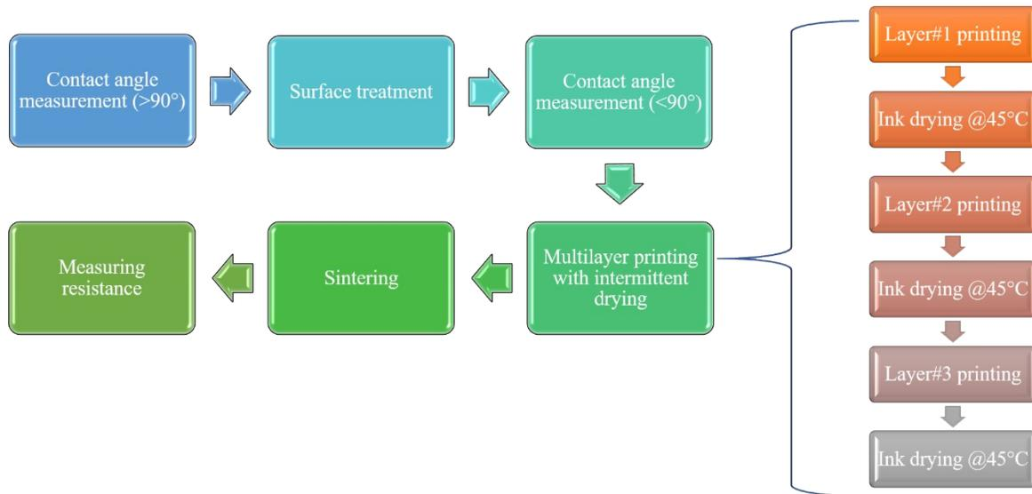
Figure 1. Fabrication process flow.
