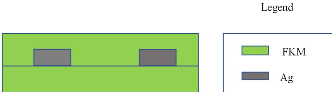
Figure 3. Silver pattern printed on/and encapsulated with FKM.
