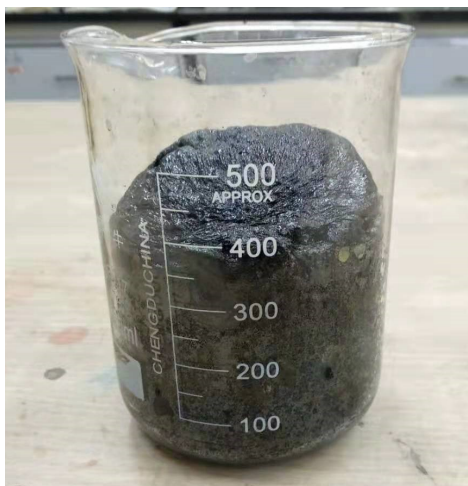
Fig. S2 The solid powder after reaction using CA (200 g), \text{CaCl}_2 (200 g) and urea (400 g) as precursors.
