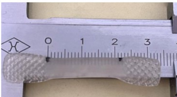
Figure S5 Length difference between two marked points: (a) the original KCPU-3 and (b) the cooled KCPU-3 after stress relaxation at 90 °C
