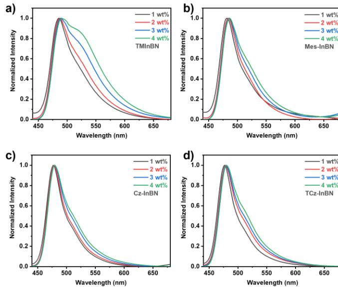
**Figure S5.** Normalized emission spectra of a) TMInBN, b) Mes-InBN, c) Cz-InBN, and d) TCz-InBN doped in mCPBC films with different dopant concentrations. mCPBC: 9-(3-(9H-carbazol-9-yl)phenyl)-9H-3,9'-bicarbazole.
