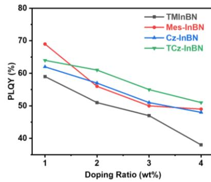
**Figure S7.** The PLQYs of TMInBN, Mes-InBN, Cz-InBN, and TCz-InBN at different dopant concentrations (in mCPBC).
