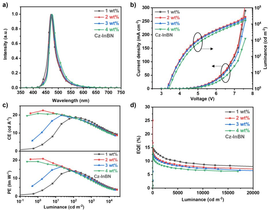
**Figure S16.** (a) EL spectra, (b) current density and luminance versus voltage, (c) current efficiency (CE) and power efficiency (PE) versus luminance, and (d) external quantum efficiency versus luminance curves of OLED devices based on Cz-InBN.
