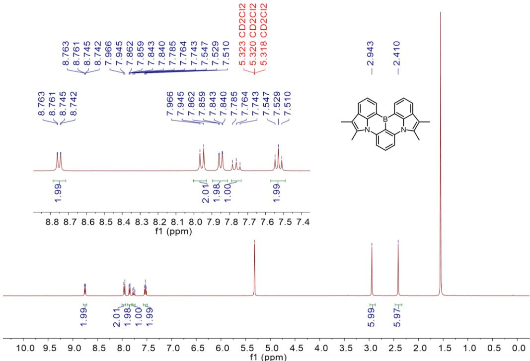
**Figure S22.**  $^1\text{H}$  NMR spectrum of **TMInBN** (400 MHz,  $\text{CD}_2\text{Cl}_2$ , 298 K).
