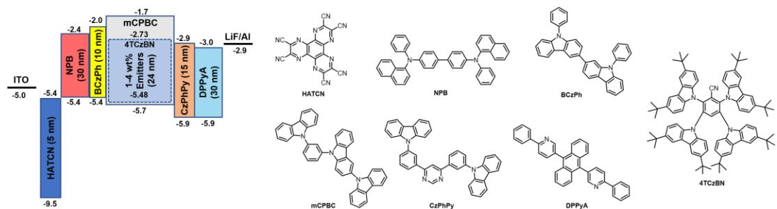
**Figure S12.** The energy diagrams of the device and the molecular structures of the materials used in the device fabrication.
