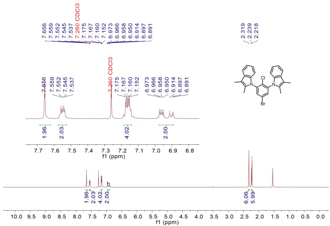
**Figure S24.**  $^1\text{H}$  NMR spectrum of **5** (400 MHz,  $\text{CDCl}_3$ , 298 K).
