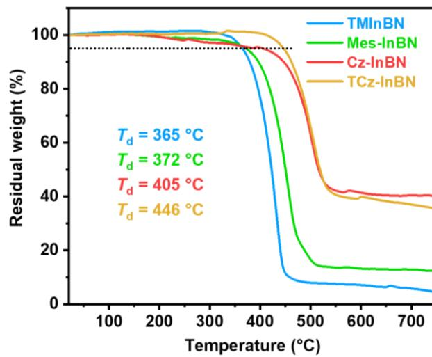
**Figure S1.** TGA curves of TMInBN, Mes-InBN, Cz-InBN, and TCz-InBN at a heating rate of  $10\text{ }^{\circ}\text{C min}^{-1}$  under a nitrogen atmosphere. Decomposition temperature ( $T_d$ ): 5% weight loss.
