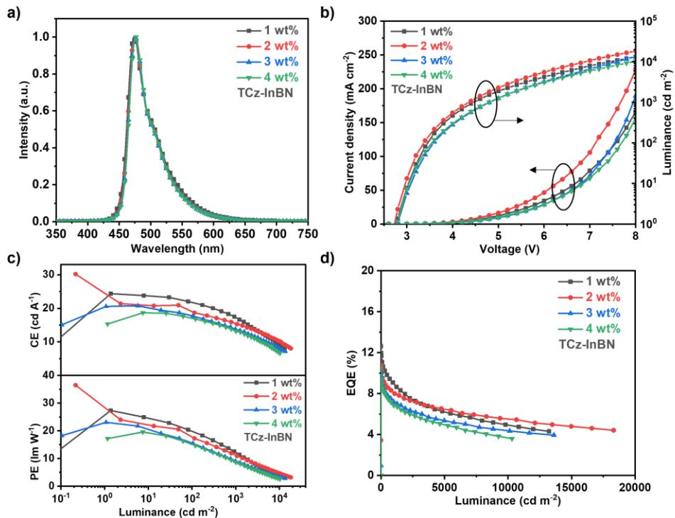
**Figure S17.** (a) EL spectra, (b) current density and luminance versus voltage, (c) current efficiency (CE) and power efficiency (PE) versus luminance, and (d) external quantum efficiency versus luminance curves of OLED devices based on TCz-InBN.
