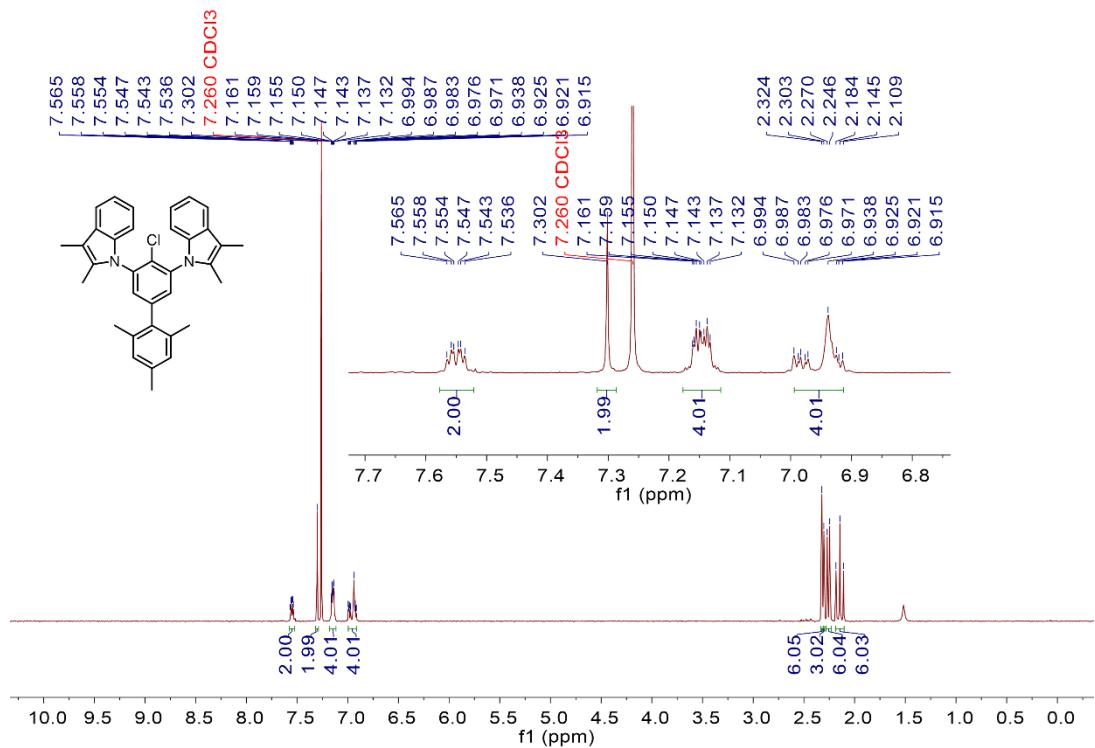
**Figure S26.**  $^1\text{H}$  NMR spectrum of **6a** (400 MHz,  $\text{CDCl}_3$ , 298 K).
