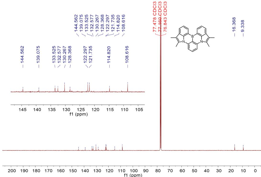
**Figure S23.**  $^{13}\text{C}$  NMR spectrum of **TMInBN** (101 MHz,  $\text{CDCl}_3$ , 298 K).
