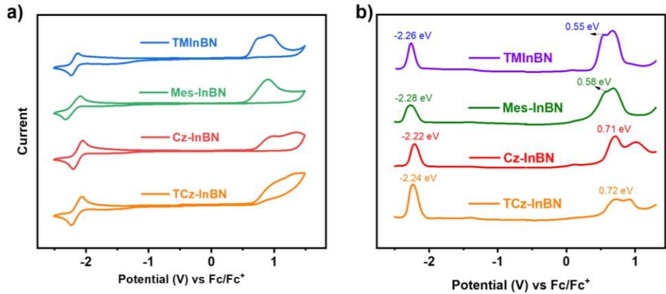
**Figure S9.** a) Cyclic voltammograms (scan rate: 100 mV s<sup>-1</sup>) and b) differential pulse voltammograms of TMInBN, Mes-InBN, Cz-InBN, and TCz-InBN in THF (1 mM) at room temperature with 0.1 M *n*-Bu<sub>4</sub>NPF<sub>6</sub> as supporting electrolyte and ferrocene as an external standard.
