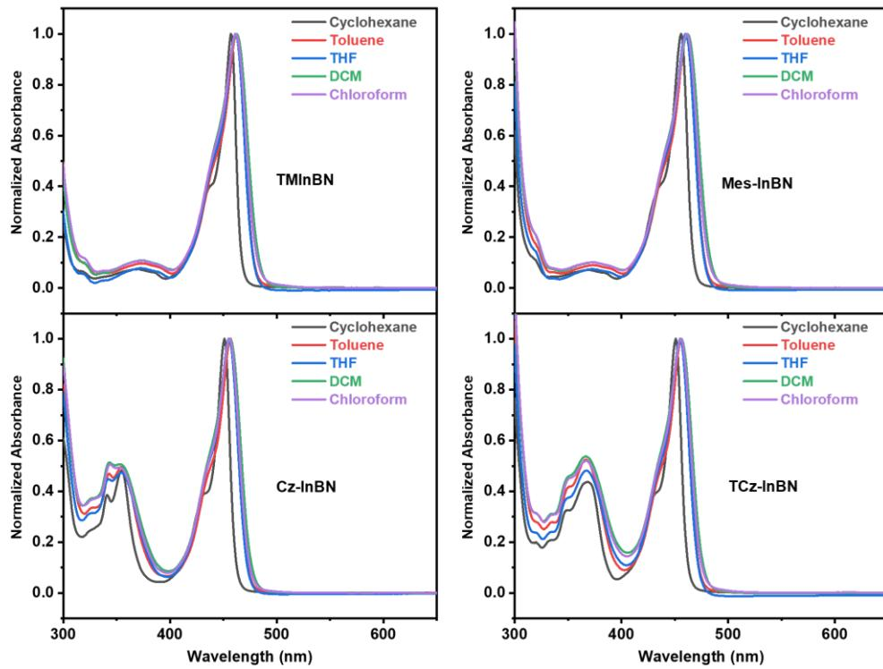
Figure S2. UV-vis absorption spectra of TMInBN, Mes-InBN, Cz-InBN, and TCz-InBN in different solvents ( $1 \times 10^{-5}$  M).
