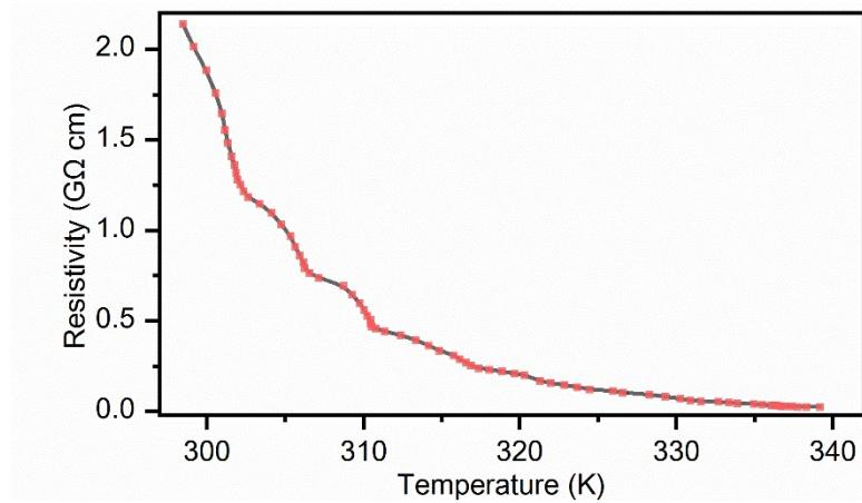
**Figure S9.** Plot of electrical resistivity versus temperature for  $\mathbf{1}\cdot\mathbf{5}\text{H}_2\text{O}$ . The measurement was performed on a pressed pellet attached to silver wires with silver paste contacts. Heating was carried out in an oil bath at a heating rate of  $3\text{ K min}^{-1}$ .
