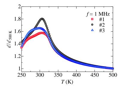
Figure S1 Sample dependence of the real part ( $\epsilon$ ') of the dielectric permittivity. Sample #1 and #2 are from same batch, and Sample #3 is from another batch. Sample #2 is also shown in the main text. The ratio between main peak around 310 K and subpeak around 270 K strongly depends on the test pellet even when the samples come from the same batch.
