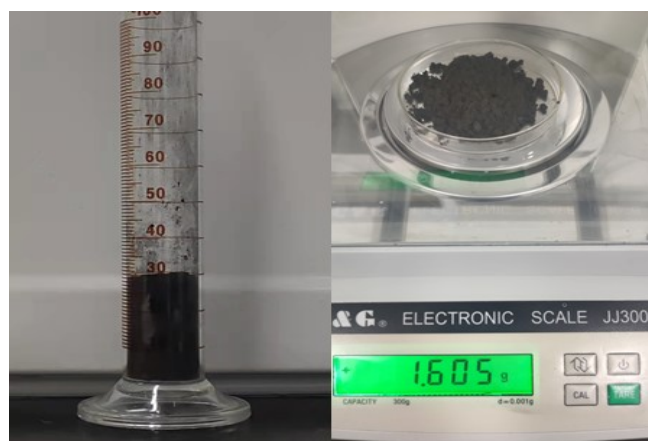
Fig. 1S Density measurement of void@C
