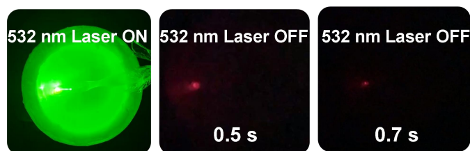
Figure S28. Photographs of R_1 -MeOBP-0.01% powders at 77 K under 532 nm laser and after removal of the laser.
