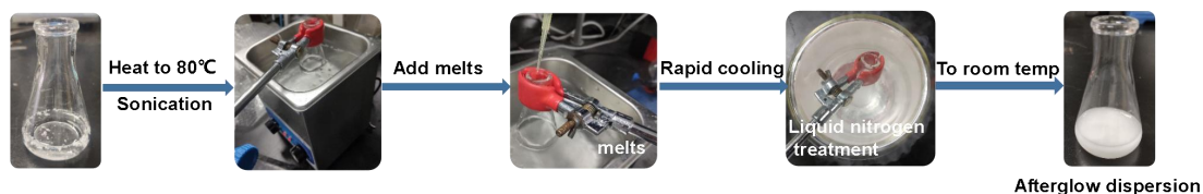
Figure S35. Procedures to prepare afterglow dispersion.
