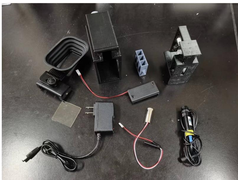
**Fig. S4** The real photographs of the main parts of smartphone-integrated analytical platform.
